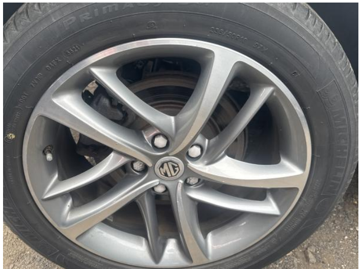
6: Wheel osr Scratched Up To 50mm
