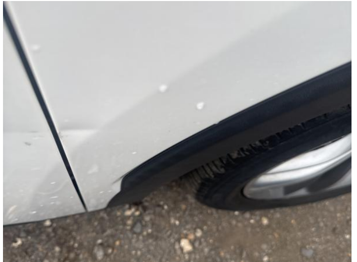
4: Wing osf Dented Between 10mm + 30mm
