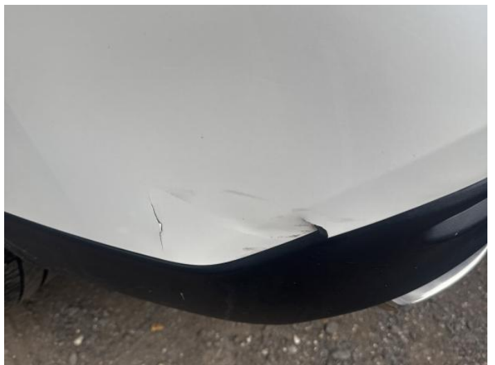
8: Bumper Rear Cracked Over 25mm
