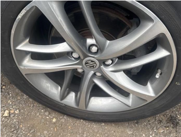
3: Wheel osf Scratched Over 50mm
