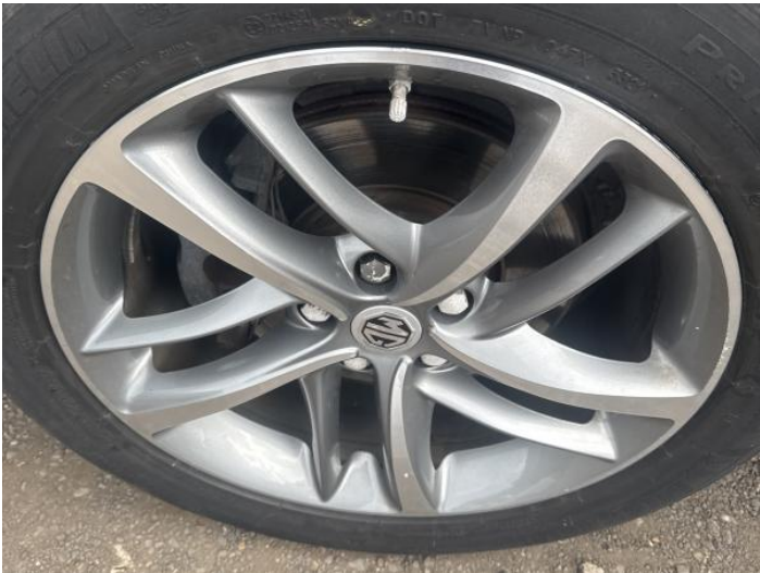
11: Wheel nsf Scratched Over 50mm
