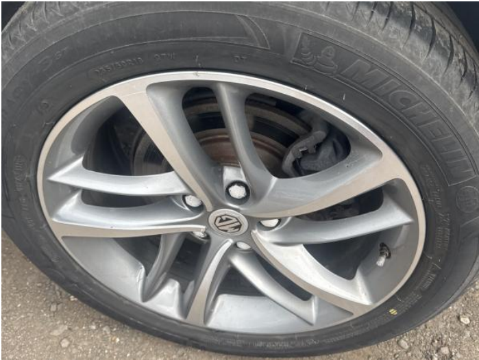
9: Wheel nsr Scratched Up To 50mm
