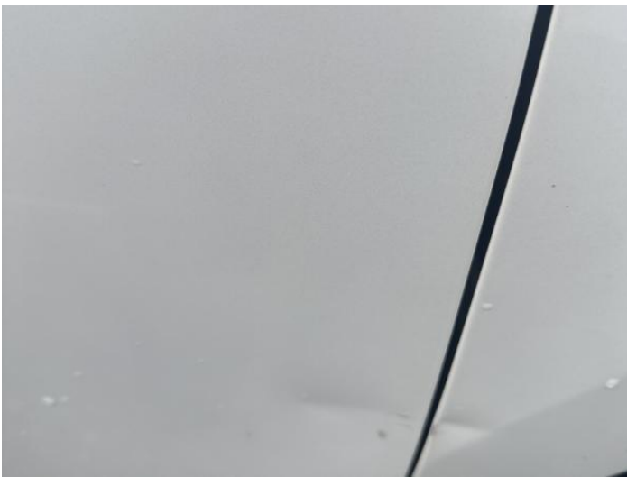
5: Door osf Dented Over 30mm
