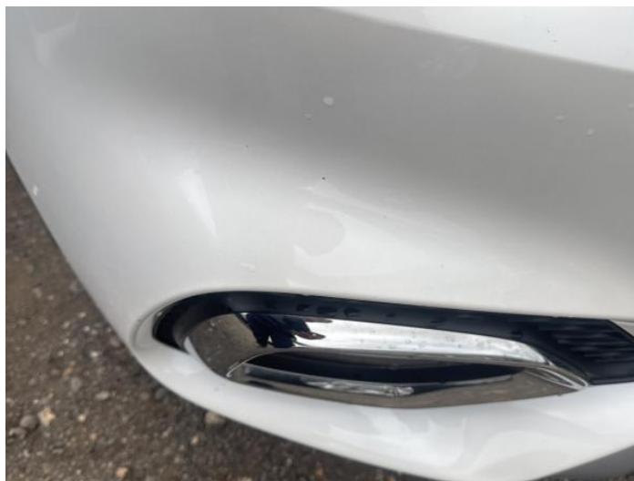
2: Bumper Front Chipped Multiple Chips
