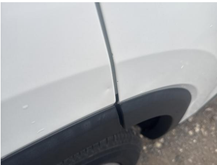
7: Qtr Panel osr Dented 2 Or Less UpTo 10mm
