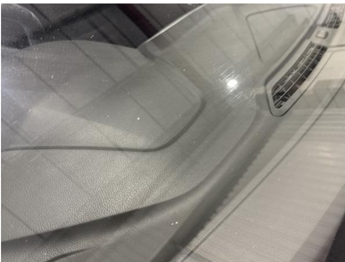
19: Screen Front Chipped UpTo 10mm
