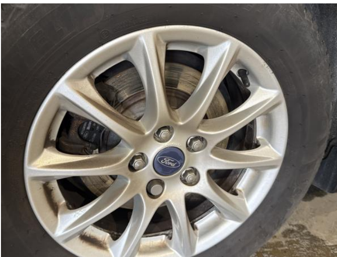
13: Wheel osr Corroded Light
