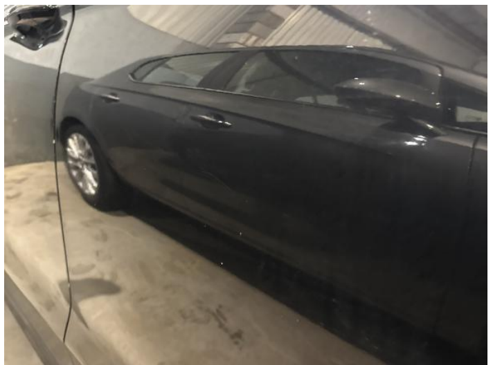
8: Door nsr Scratched Over 25mm Thru Paint
