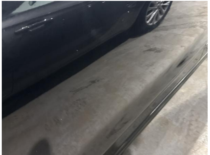
6: Door nsf Dented Over 30mm
