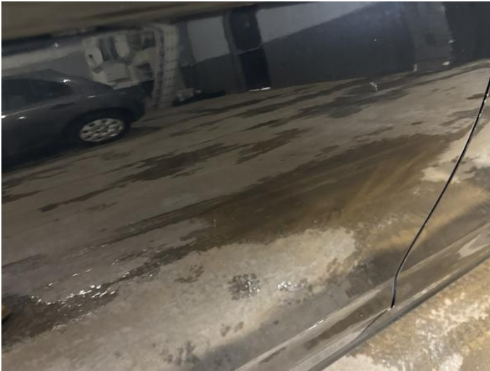
15: Door osr Scratched UpTo 25mm Thru Paint
