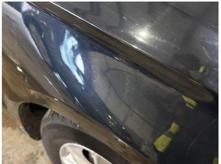
18: Wing osf Scratched UpTo 25mm Thru Paint
