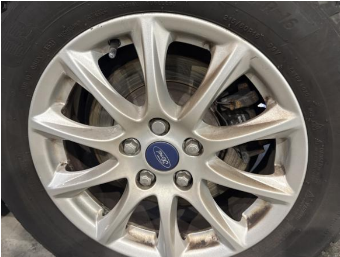
9: Wheel nsr Corroded Light
