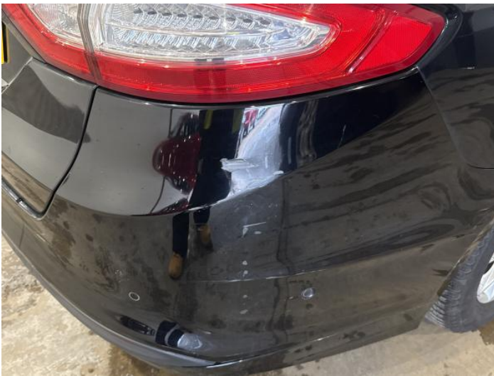
11: Bumper Rear Scratched 25 to 100mm Thru Paint
