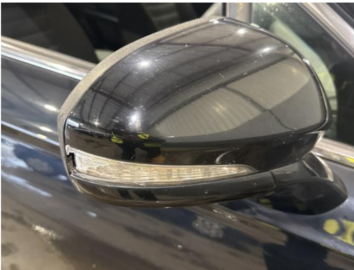
17: Flasher Side Repeater os Broken Replace
