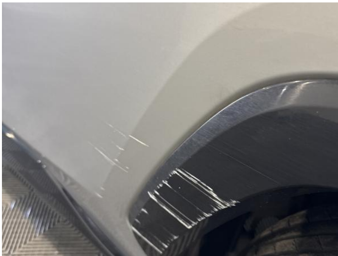
5: Door nsr Scratched Over 25mm Thru Paint
