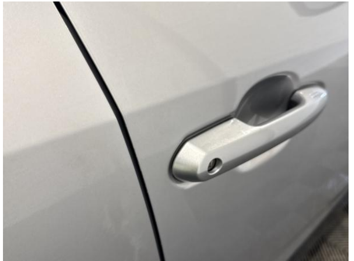
12: Door osf Chipped Edge Chip
