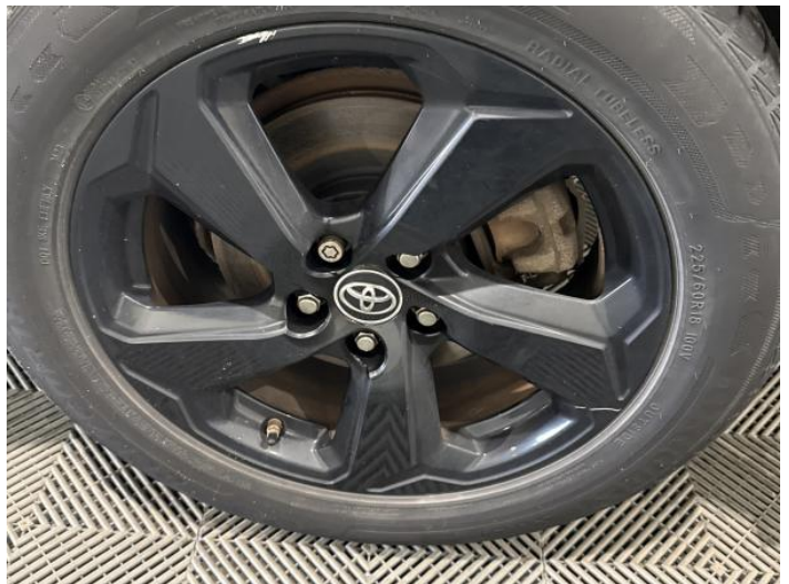
6: Wheel nsr Scratched Up To 50mm
