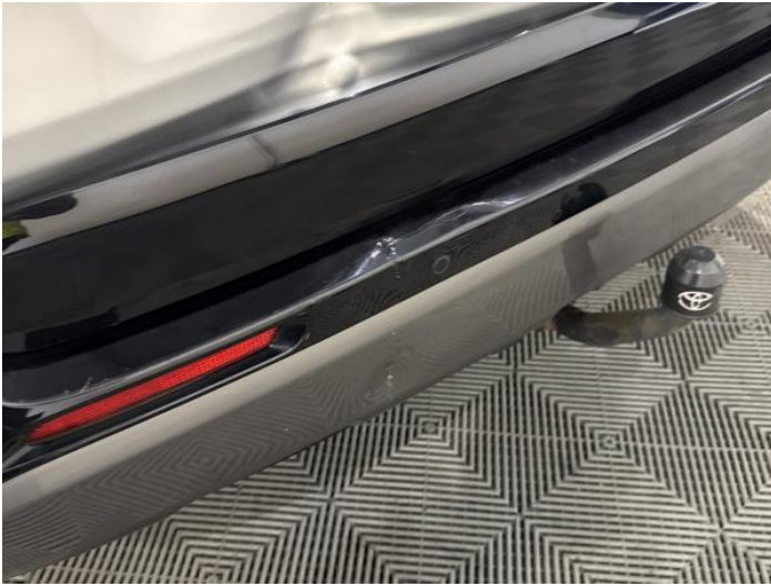
9: Bumper Rear Dented Over 30mm
