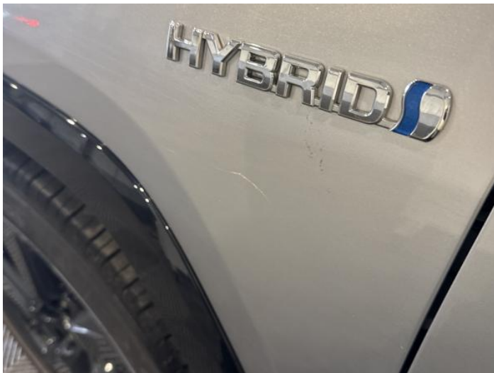
3: Wing nsf Scratched Over 25mm Thru Paint
