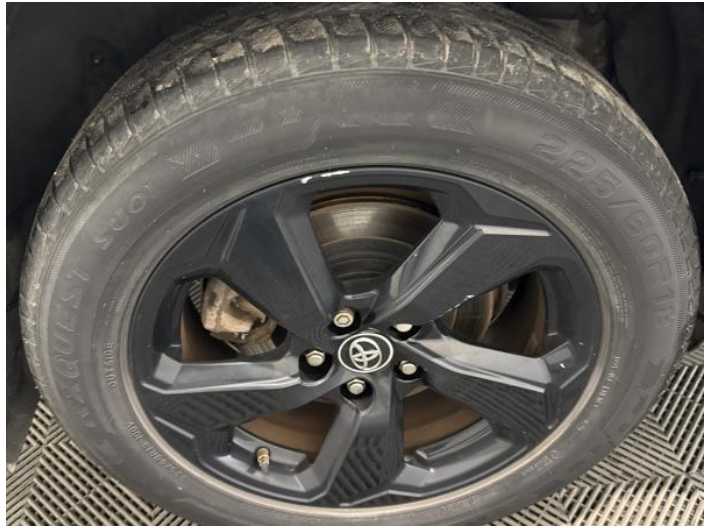
10: Wheel osr Scratched Up To 50mm
