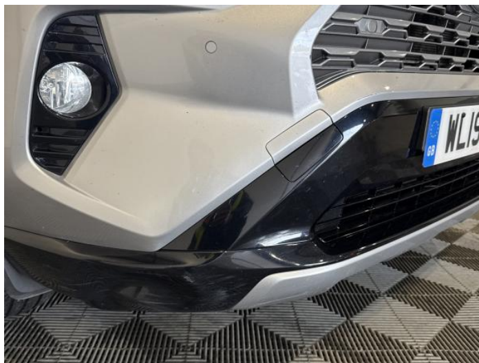
2: Bumper Front Dented With Paint Damage
