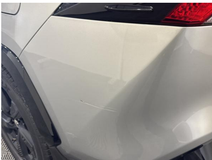
7: Bumper Rear Moulding Scratched (Painted) Over 25mm Thru Paint
