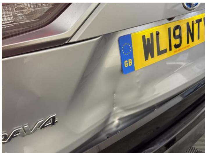
8: Tailgate Dented With Paint Damage
