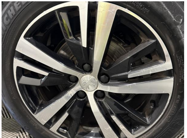
6: Wheel nsr Corroded Light
