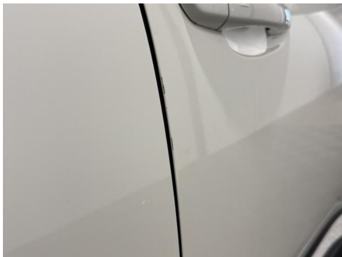
10: Door osf Chipped Edge Chip
