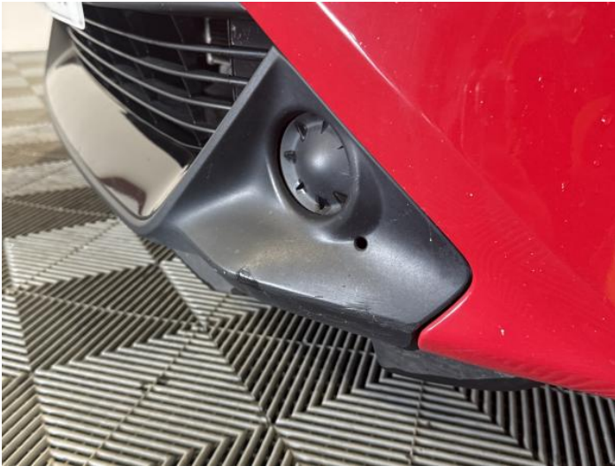
3: Bumper Front Moulding Scuffed (Unpainted) Over 100mm
