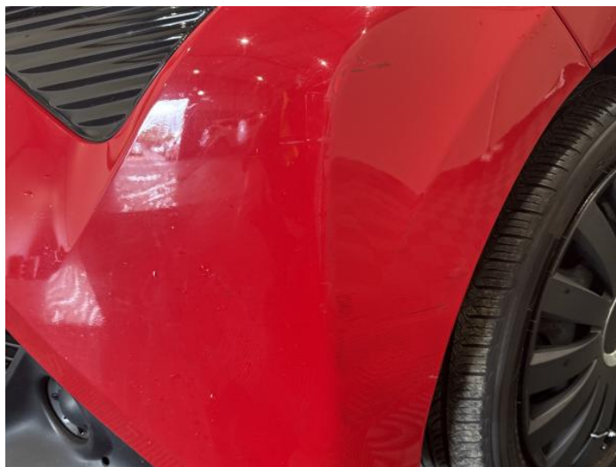
2: Bumper Front Scratched 25 to 100mm Thru Paint
