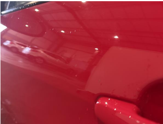
5: Door nsf Dented Over 2 UpTo 10mm
