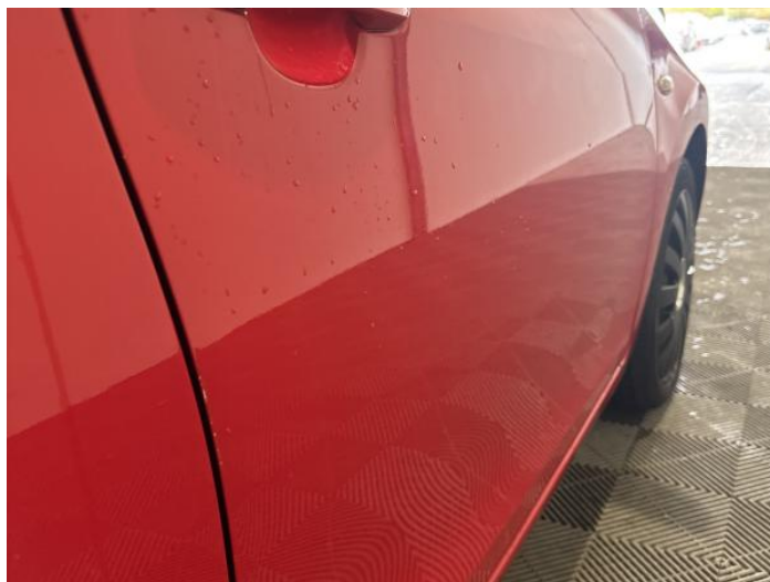
10: Door osf Dented Between 10mm + 30mm
