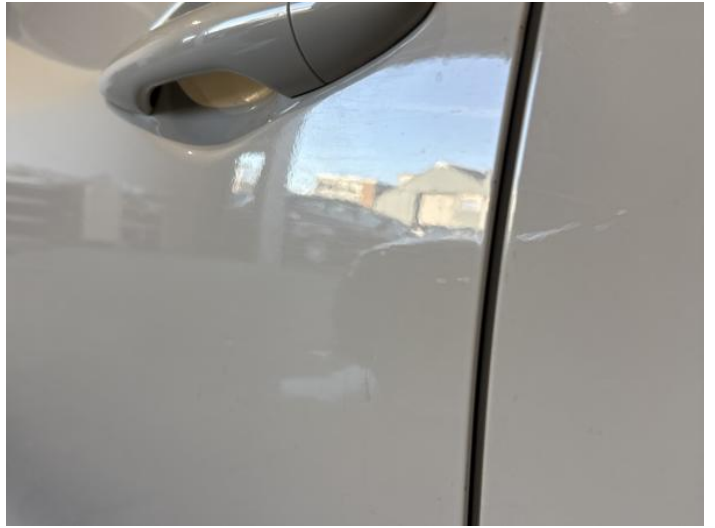
4: Door nsf Scratched UpTo 25mm Thru Paint
