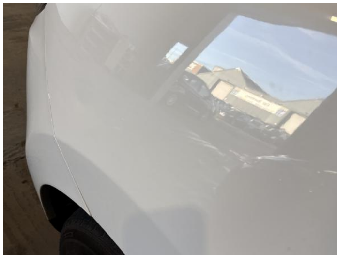
16: Wing nsf Dented Over 30mm
