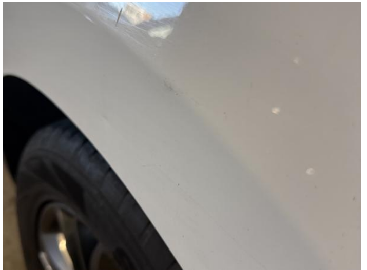
6: Qtr Panel nsr Dented Between 10mm + 30mm
