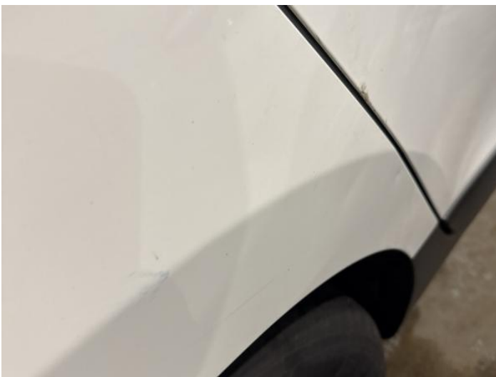
7: Qtr Panel osr Dented Over 30mm
