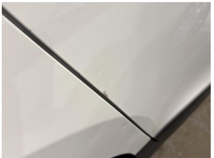
8: Door osr Scratched UpTo 25mm Thru Paint
