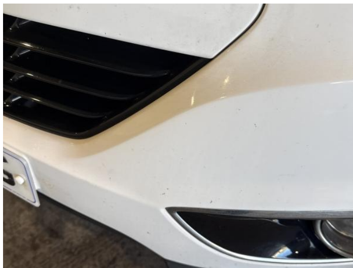
2: Bumper Front Scratched 25 to 100mm Thru Paint
