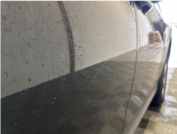
17: Door osr Dented With Paint Damage
