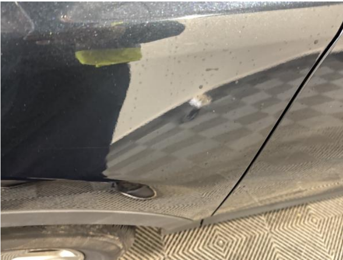
5: Wing nsf Dented Over 2 UpTo 10mm
