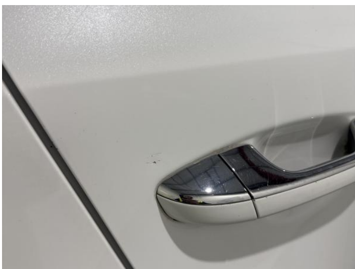
11: Door osr Scratched UpTo 25mm Thru Paint
