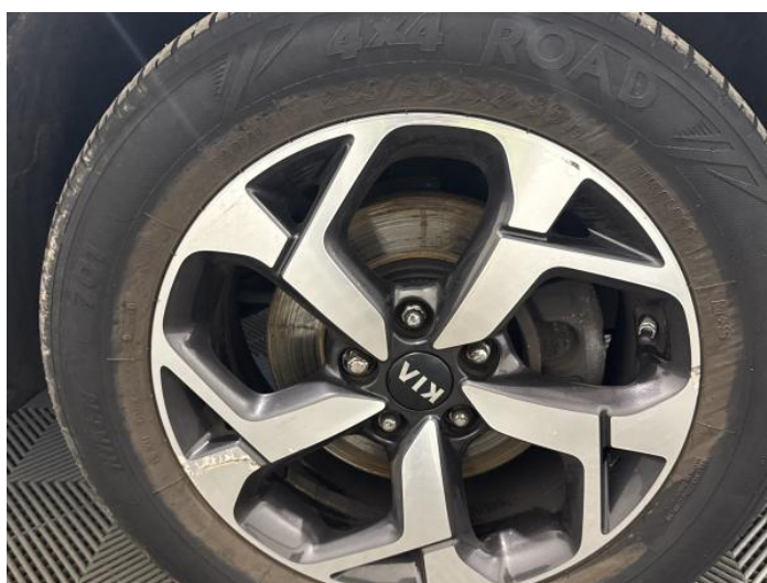
14: Wheel osf Scratched Over 50mm
