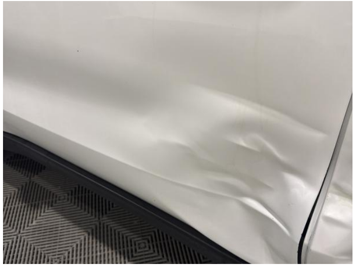
4: Door nsf Dented Over 30mm
