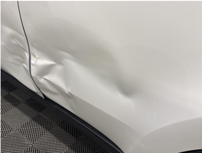
5: Door nsr Dented Over 30% Of Panel
