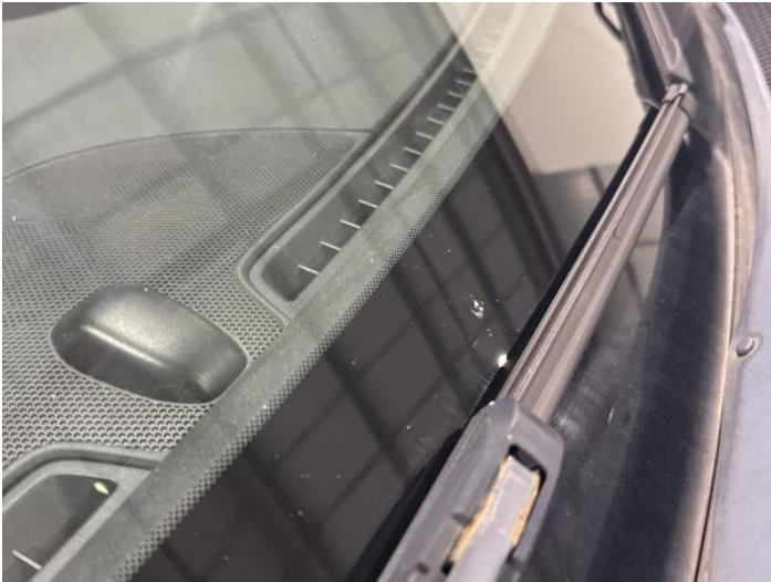
15: Screen Front Chipped UpTo 10mm
