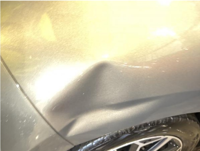
16: Qtr Panel osr Dented Over 30mm
