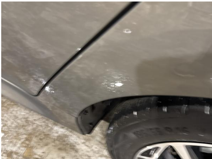
3: Qtr Panel nsr Dented Over 2 UpTo 10mm
