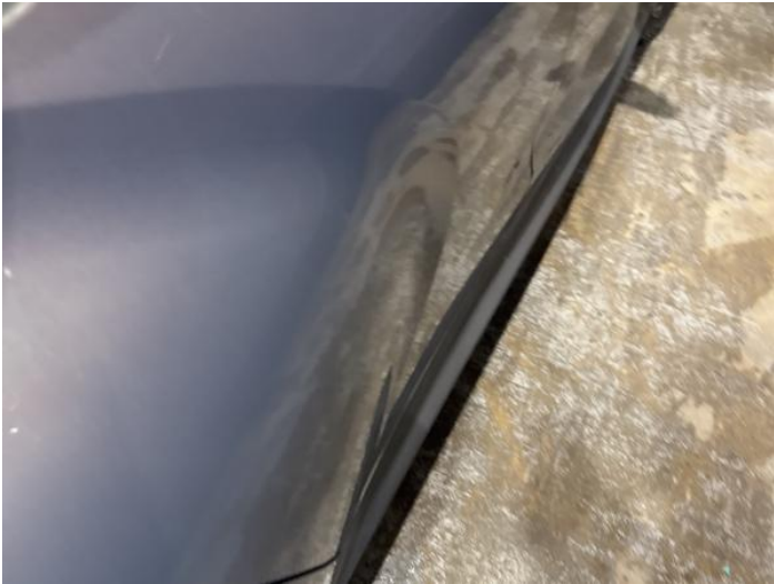
15: Door osr Dented Over 2 UpTo 10mm
