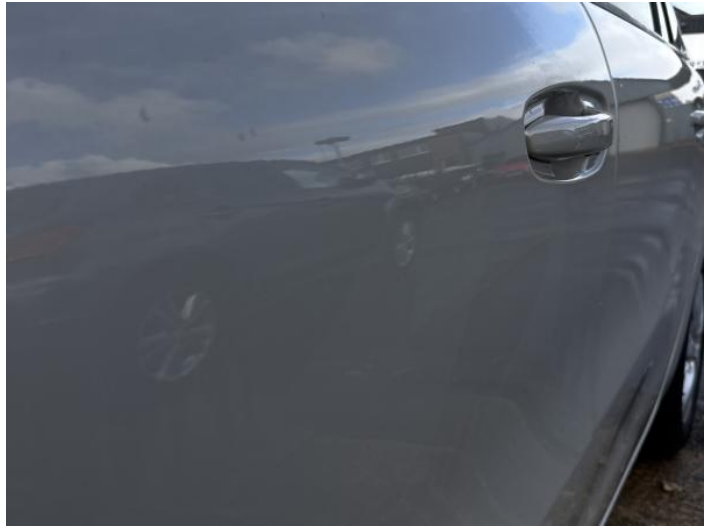
4: Door nsf Dented Between 10mm + 30mm
