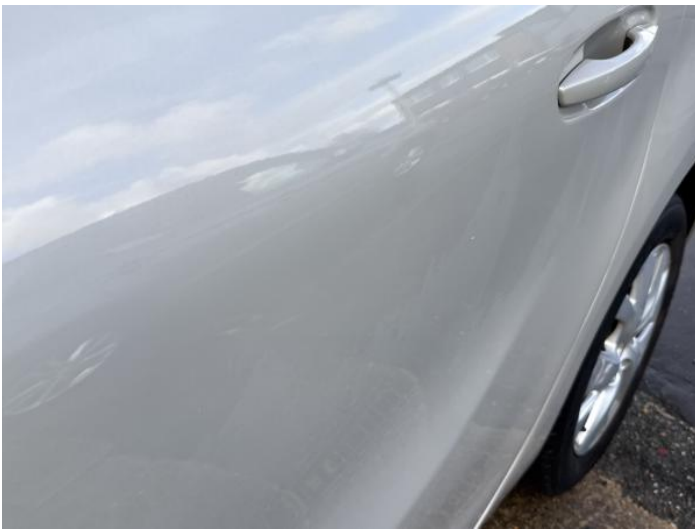
5: Door nsr Dented Between 10mm + 30mm
