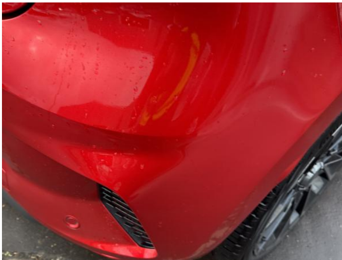
9: Bumper Rear Chipped Multiple Chips
