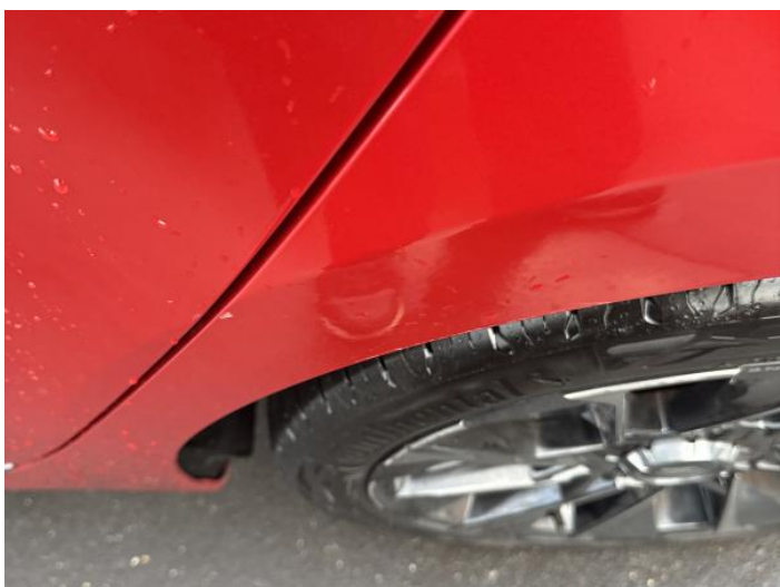
7: Qtr Panel nsr Chipped 1 To 5
