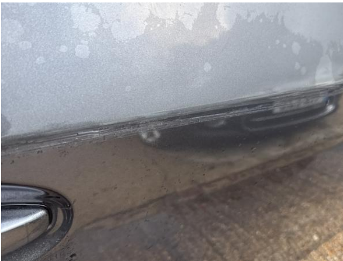
5: Door osr Scratched Over 25mm Thru Paint
