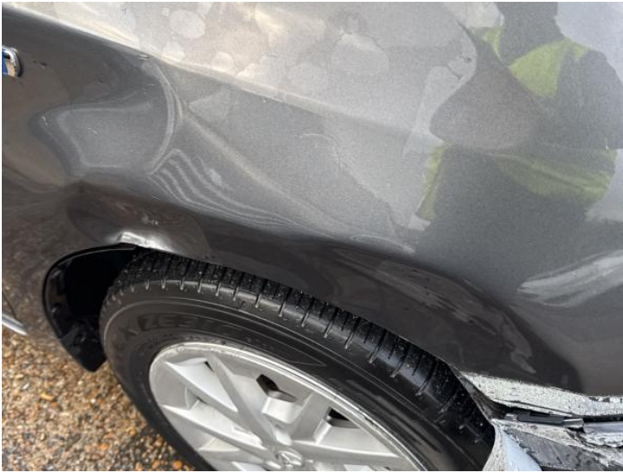
3: Wing osf Dented Over 30% Of Panel
