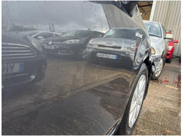
4: Door osf Dented Over 30mm
