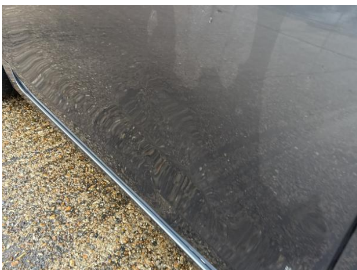
11: Door nsf Dented Over 30mm
