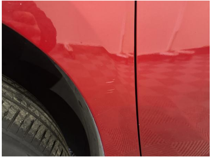
4: Wing nsf Scratched Over 25mm Thru Paint
