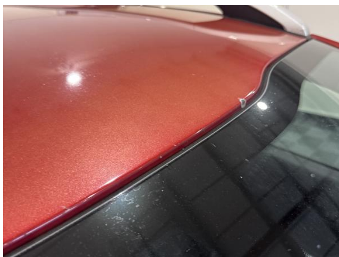
18: Roof Chipped Over 5mm
