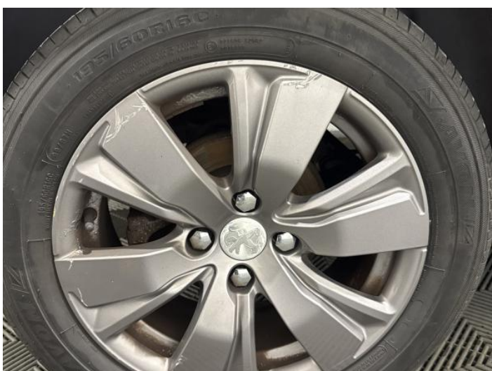
13: Wheel osr Scratched Over 50mm
