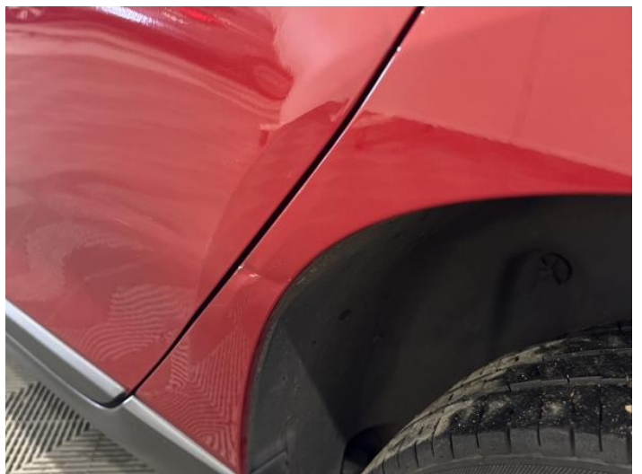
8: Qtr Panel nsr Dented Over 30mm
