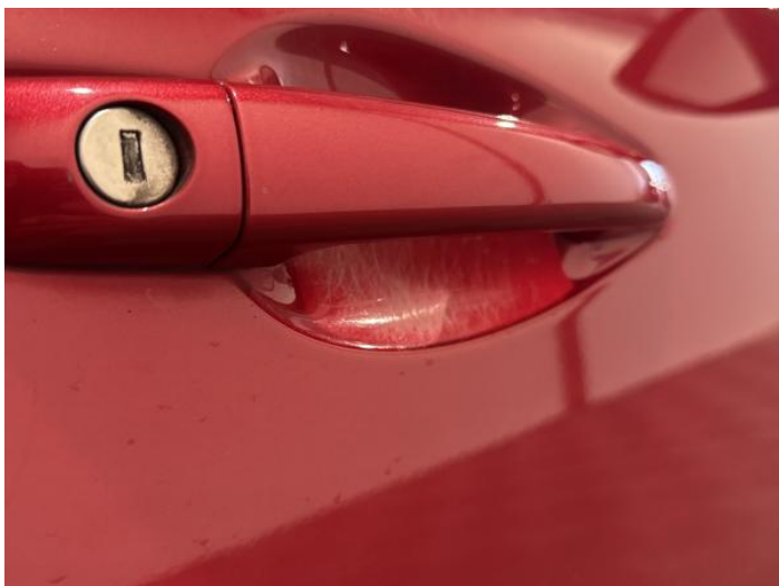
15: Door osf Scratched Over 25mm Thru Paint
