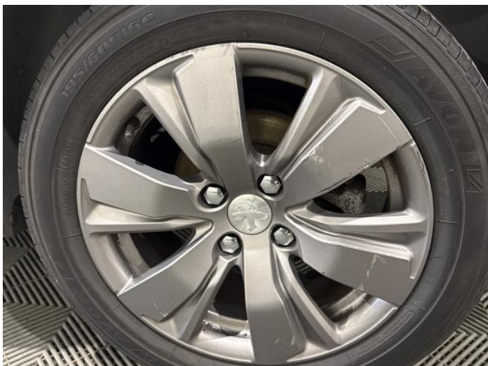
9: Wheel nsr Scratched Over 50mm
