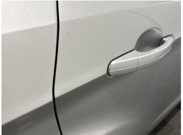
10: Door osr Chipped 1 To 5
