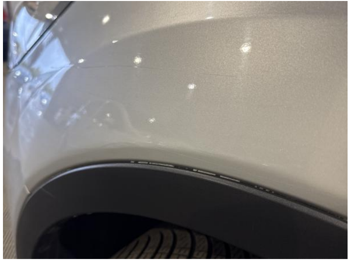
4: Wing nsf Poor Previous Repair Poor Paint
