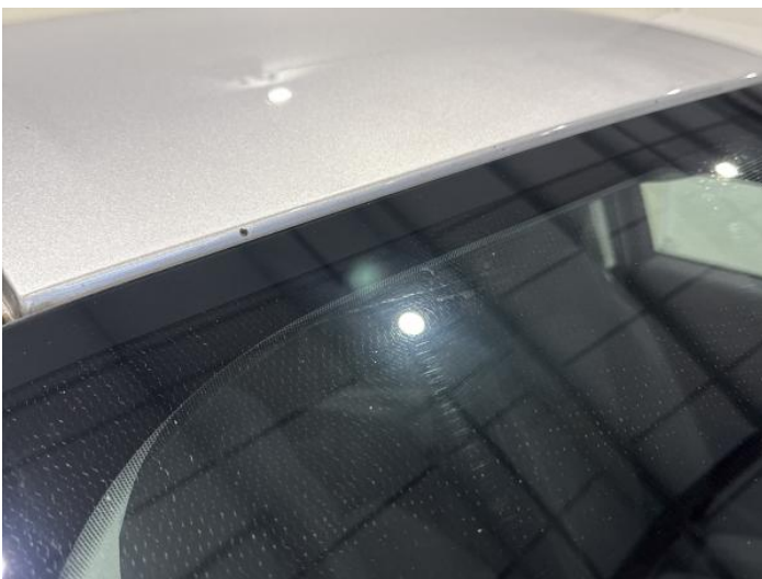
13: Roof Chipped Edge Chip
