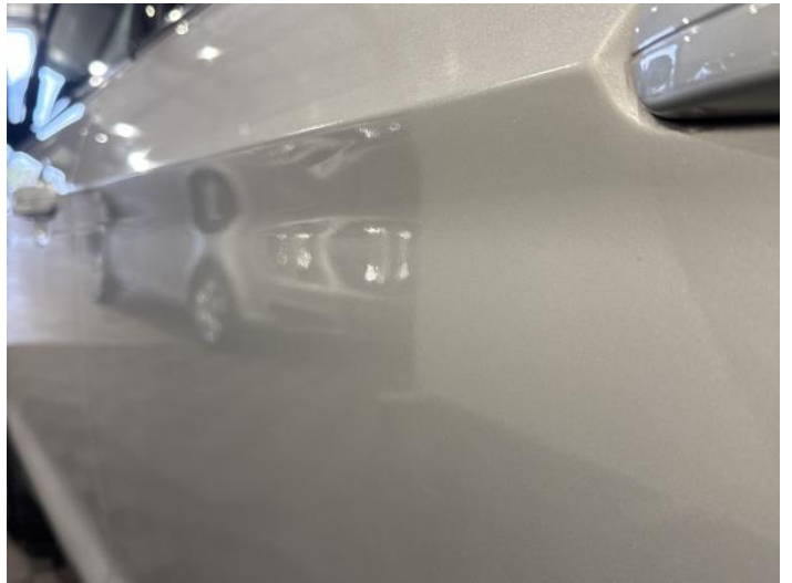
6: Door nsr Dented Over 30mm
