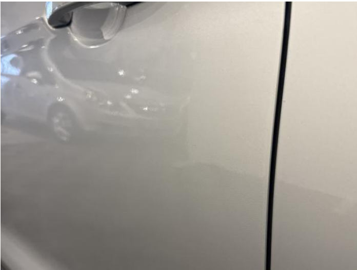
5: Door nsf Poor Previous Repair Poor Paint
