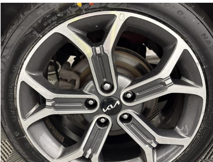
7: Wheel osr Scratched Over 50mm
