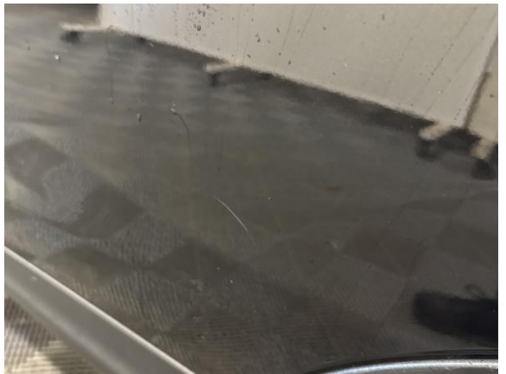
6: Door nsr Scratched Over 25mm Thru Paint
