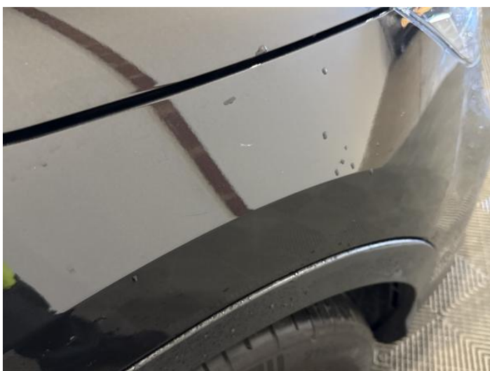
11: Wing osf Scratched UpTo 25mm Thru Paint
