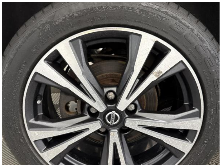
8: Wheel osr Corroded Light
