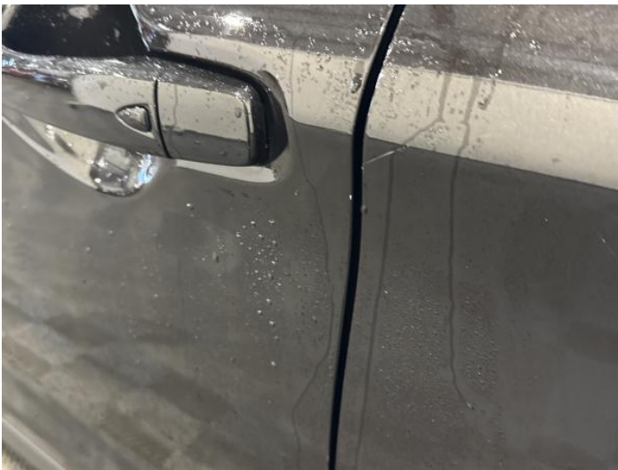
5: Door osf Chipped Edge Chip
