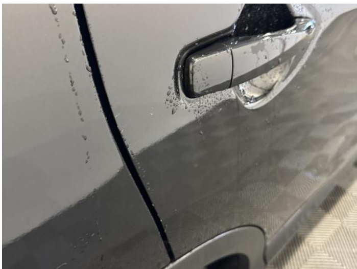
9: Door osr Chipped Edge Chip
