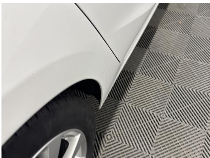
13: Qtr Panel osr Dented Over 30mm
