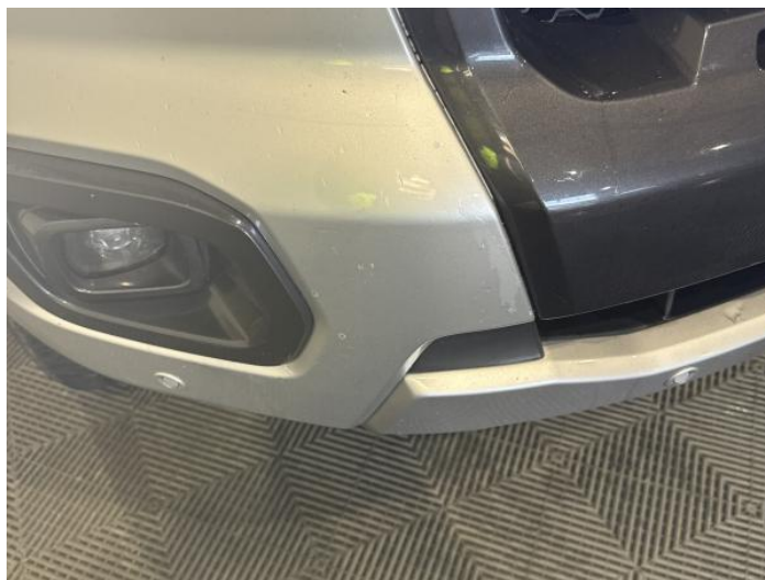
2: Bumper Front Poor Previous Repair Paint Flake
