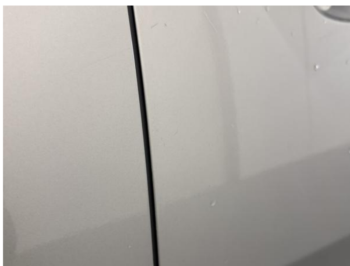
8: Door osf Scratched UpTo 25mm Thru Paint
