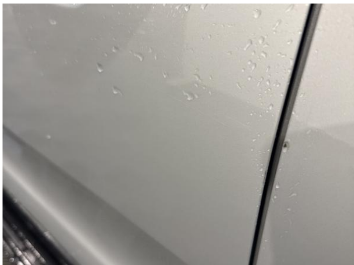
3: Door nsf Scratched Over 25mm Thru Paint
