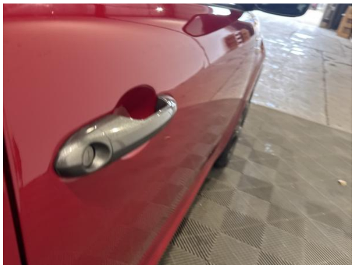
14: Door osf Dented Over 30mm
