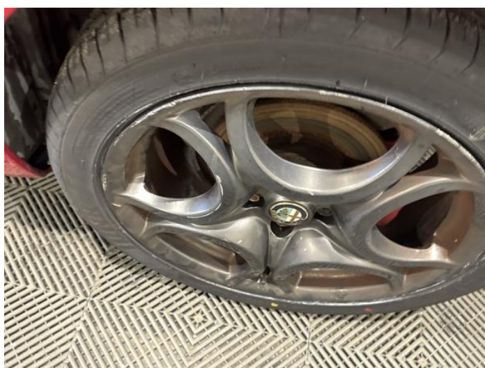
8: Wheel nsr Scratched Over 50mm
