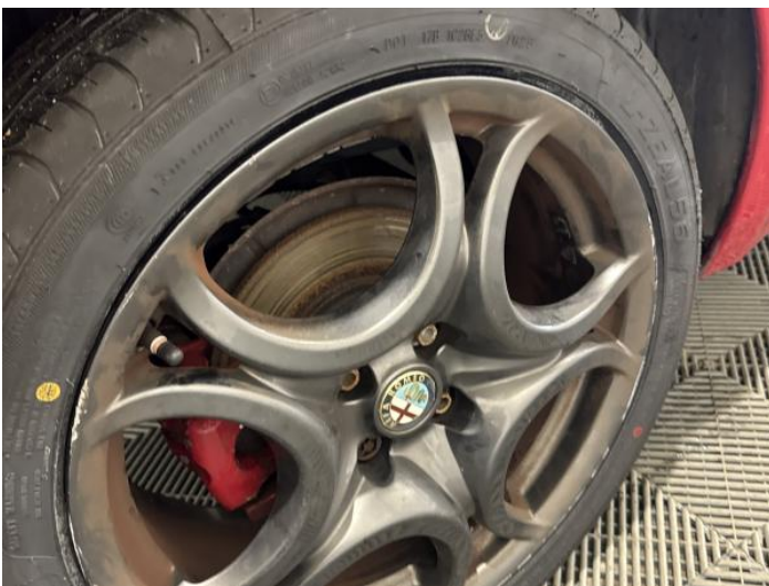
13: Wheel osr Scratched Over 50mm
