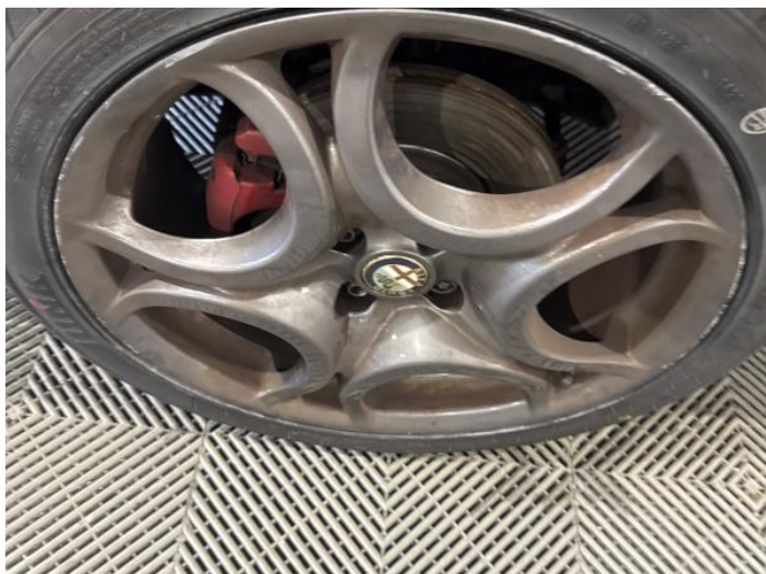
3: Wheel nsf Scratched Over 50mm
