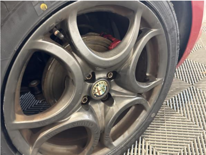
16: Wheel osf Scratched Over 50mm
