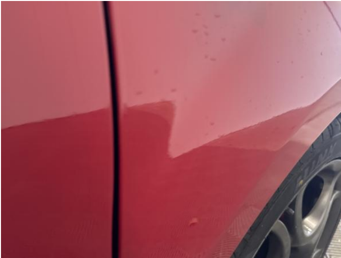
15: Wing osf Poor Previous Repair Poor Paint
