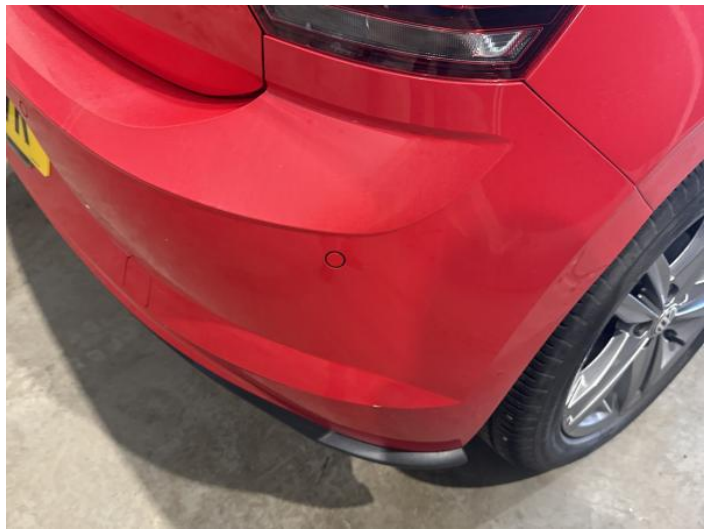
6: Bumper Rear Scratched 25 to 100mm Thru Paint
