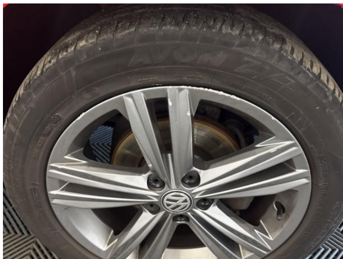
10: Wheel osf Scratched Over 50mm
