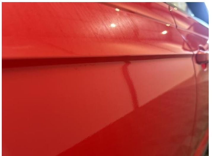
8: Door osr Scratched Over 25mm Thru Paint
