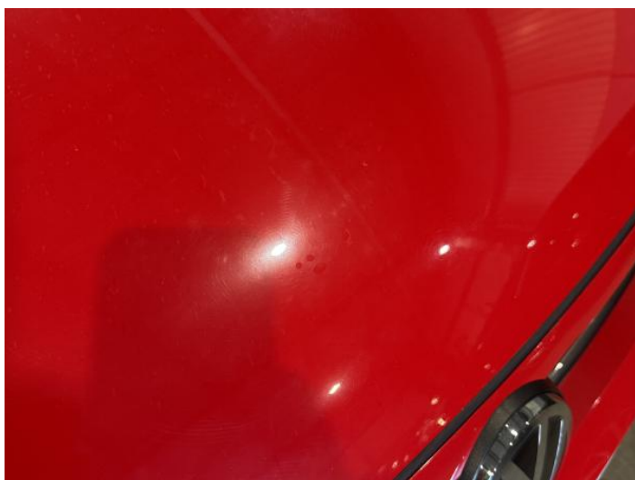
1: Bonnet Chipped Multiple Chips
