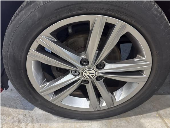
3: Wheel nsf Scratched Up To 50mm
