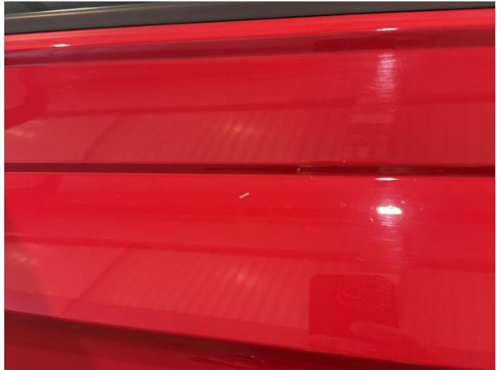
4: Door nsf Scratched UpTo 25mm Thru Paint
