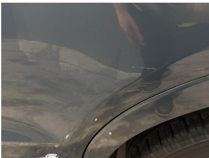
7: Door nsr Scratched Over 25mm Thru Paint
