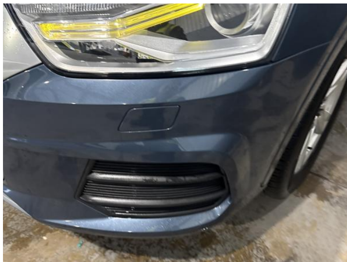
2: Bumper Front Scratched Over 100mm Thru Paint
