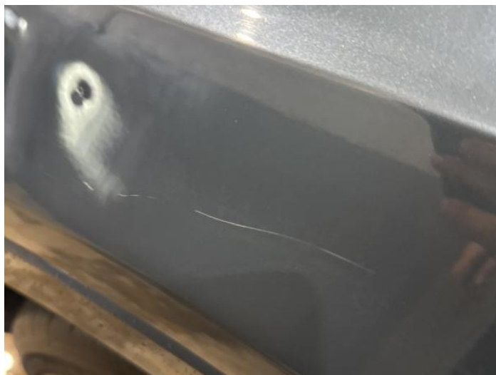
4: Wing nsf Dented With Paint Damage
