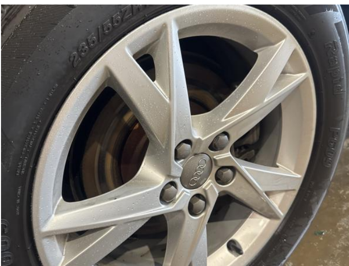
13: Wheel osr Scratched Up To 50mm
