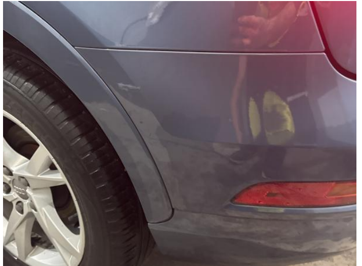
10: Bumper Rear Scratched Over 100mm Thru Paint
