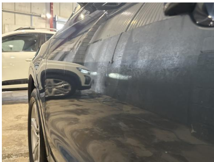
6: Door nsf Poor Previous Repair Poor Paint
