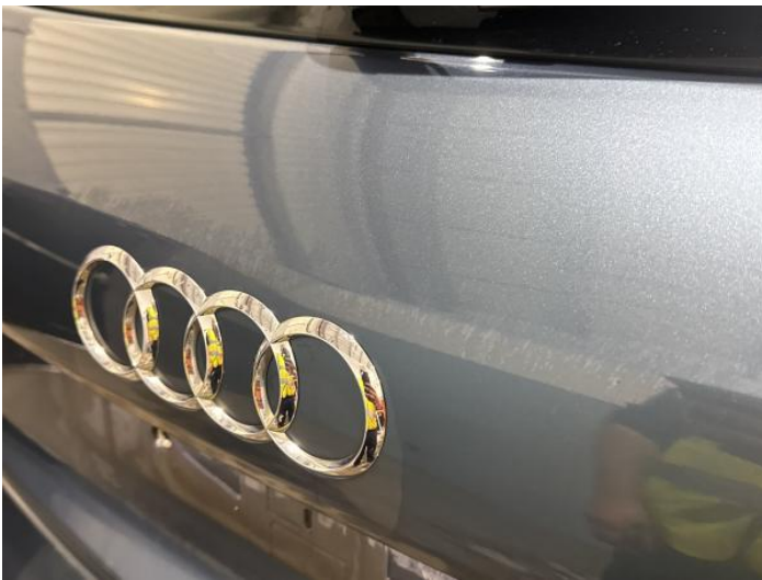
11: Boot Lid Dented 2 Or Less UpTo 10mm
