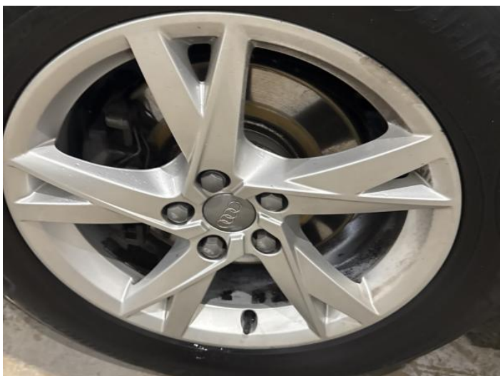
5: Wheel nsf Scratched Up To 50mm
