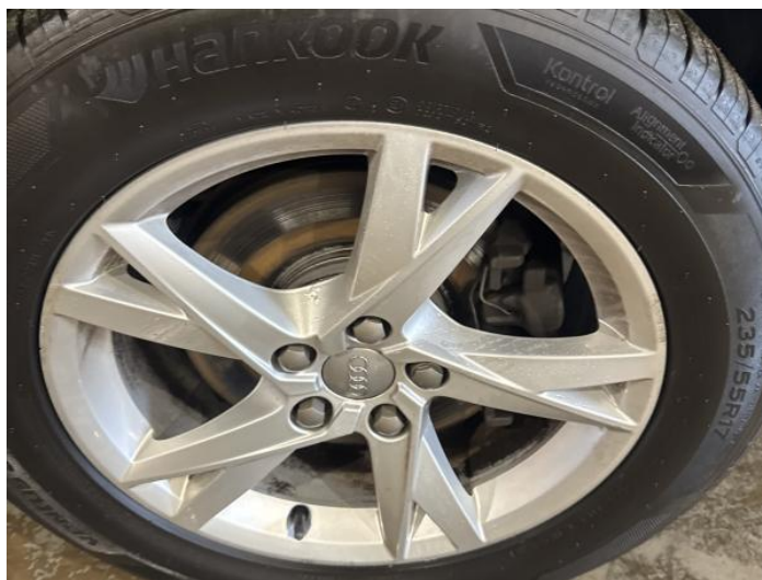
18: Wheel osf Scratched Over 50mm
