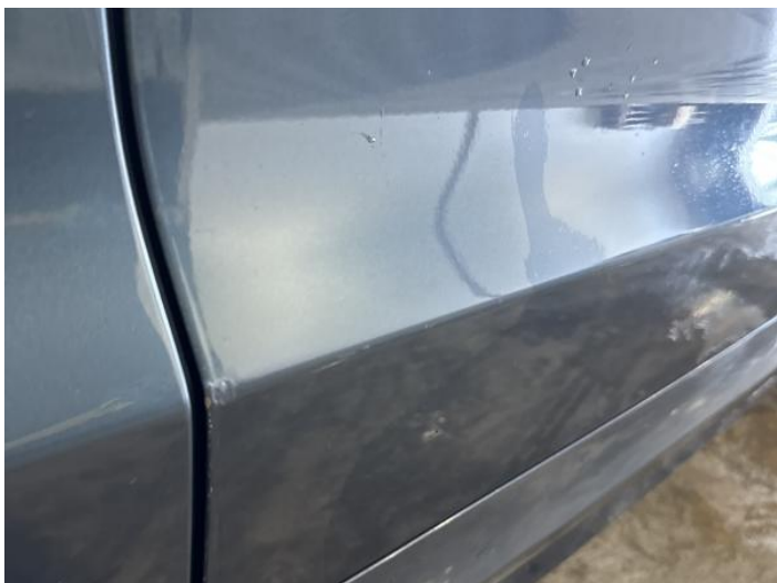
15: Door osf Chipped Edge Chip
