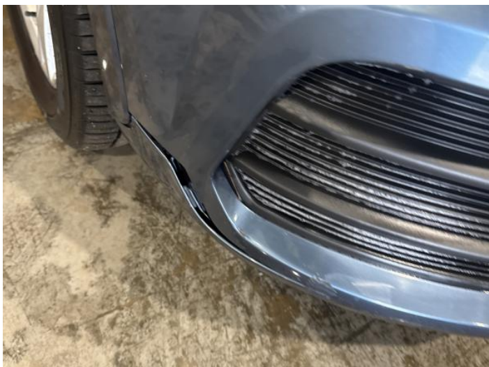
3: Bumper Front Moulding Broken Replace
