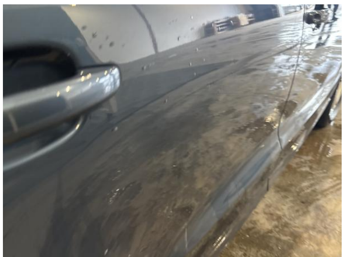
14: Door osr Dented With Paint Damage
