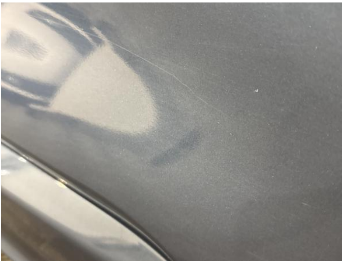
5: Door nsr Scratched Over 25mm Thru Paint
