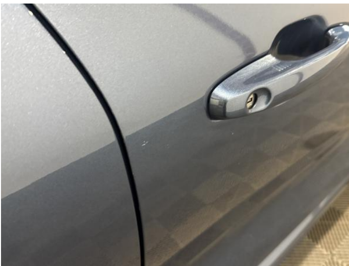
7: Door osf Scratched UpTo 25mm Thru Paint
