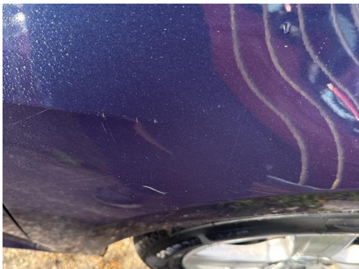
9: Wing osf Scratched UpTo 25mm Thru Paint
