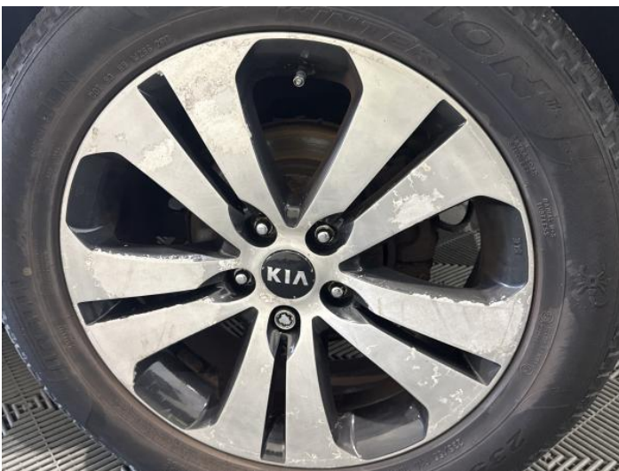
7: Wheel osr Scratched Over 50mm
