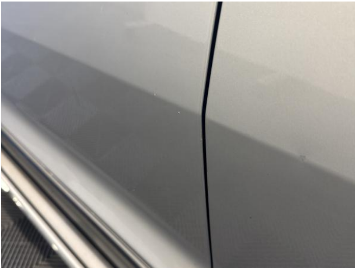
5: Door nsf Scratched Over 25mm Thru Paint
