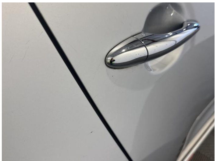
12: Door osr Scratched Over 25mm Thru Paint
