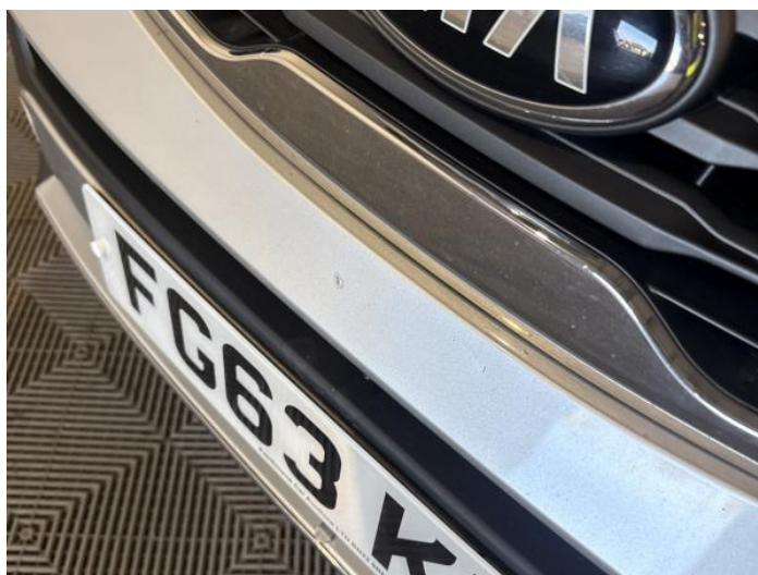
2: Bumper Front Chipped Over 5mm
