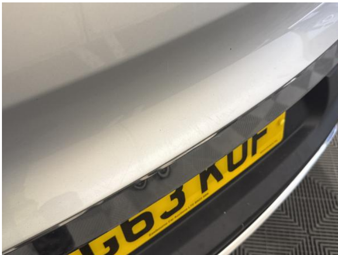
9: Tailgate Scratched UpTo 25mm Thru Paint
