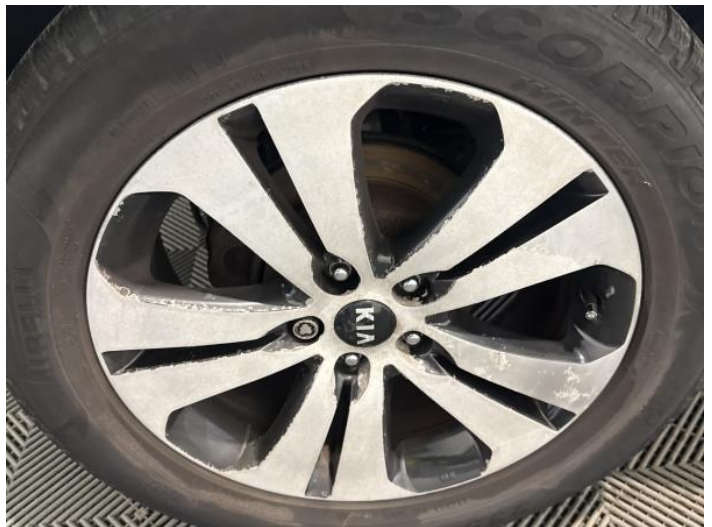
10: Wheel osr Scratched Over 50mm
