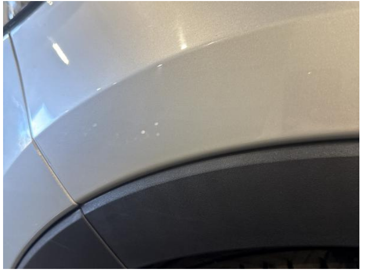
4: Wing nsf Scratched UpTo 25mm Thru Paint
