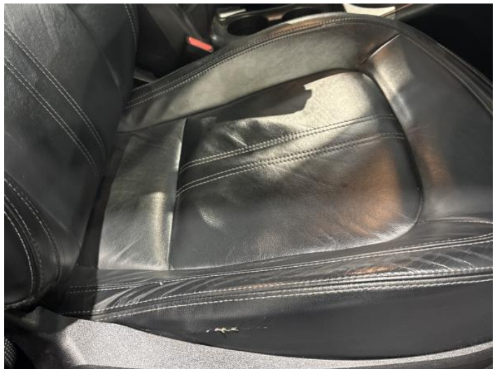
16: Seat Base Cover osf Scuffed Over 25mm
