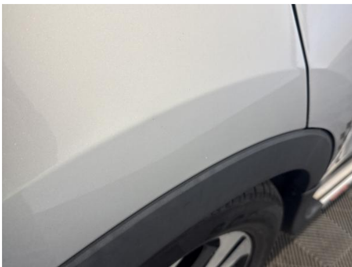
11: Qtr Panel osr Dented Between 10mm + 30mm
