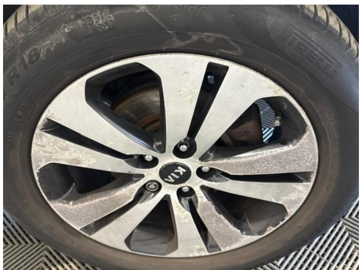
14: Wheel osf Scratched Over 50mm
