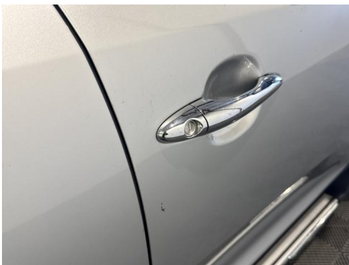
13: Door osf Scratched Over 25mm Thru Paint
