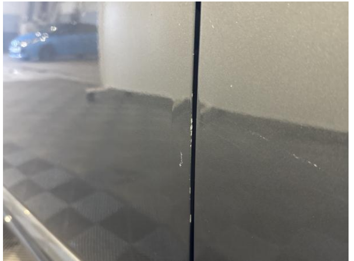
6: Door nsf Dented Over 30mm
