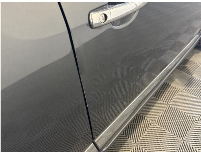
13: Door osf Dented Over 30mm
