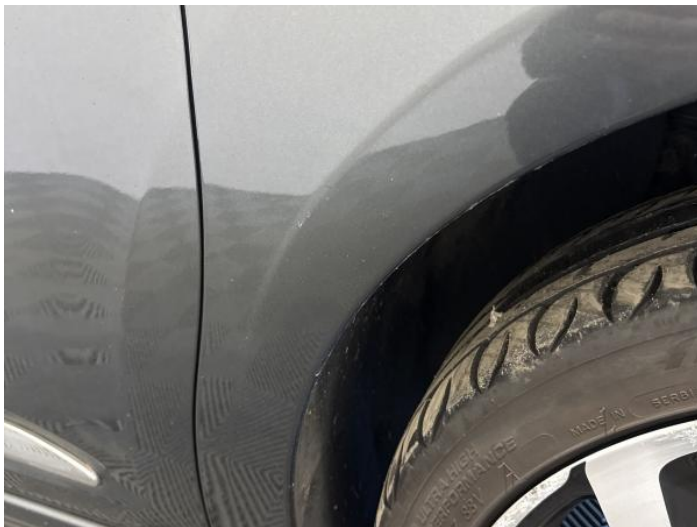
15: Wing osf Scratched UpTo 25mm Thru Paint
