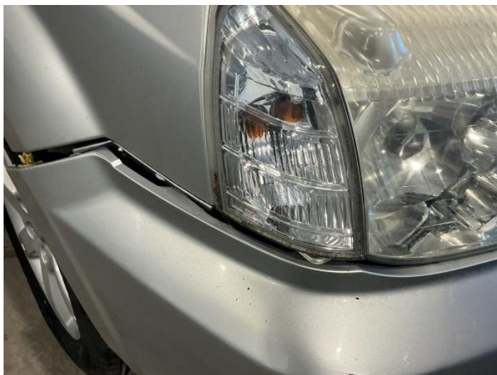
1: Bumper Front Cracked Over 25mm
