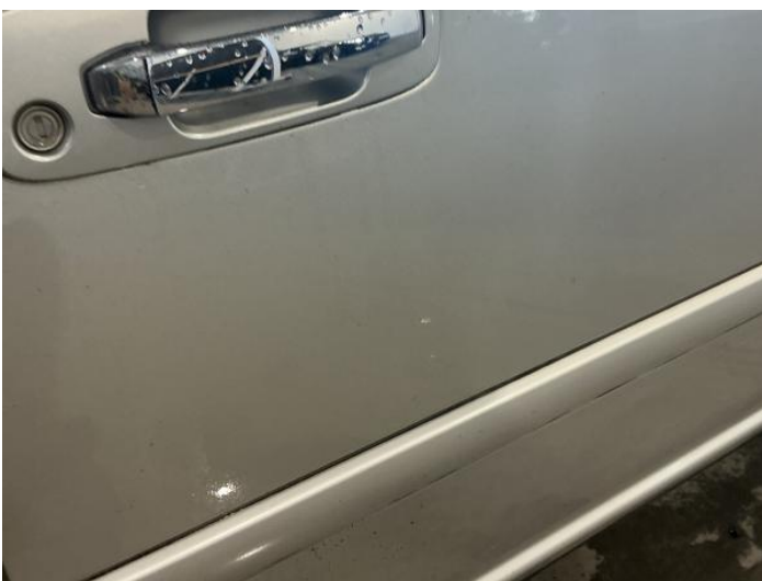
13: Door osf Poor Previous Repair Poor Paint
