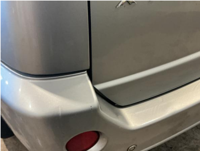
9: Bumper Rear Scratched 25 to 100mm Thru Paint
