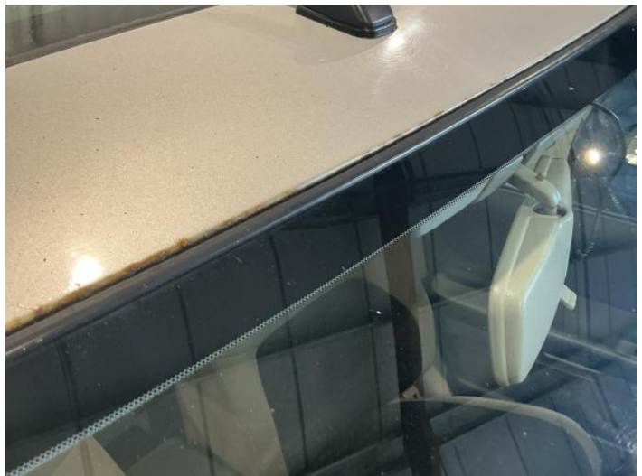
16: Roof Rusted Over 5mm
