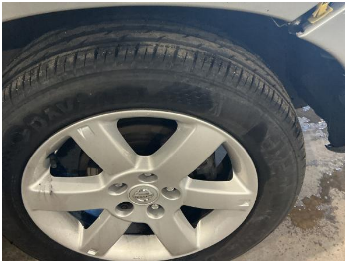
15: Wheel osf Scratched Up To 50mm
