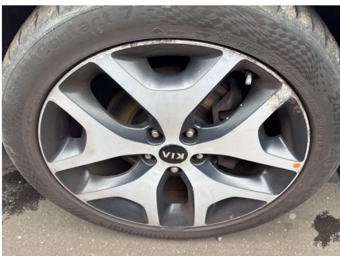
19: Wheel osf Scratched Over 50mm
