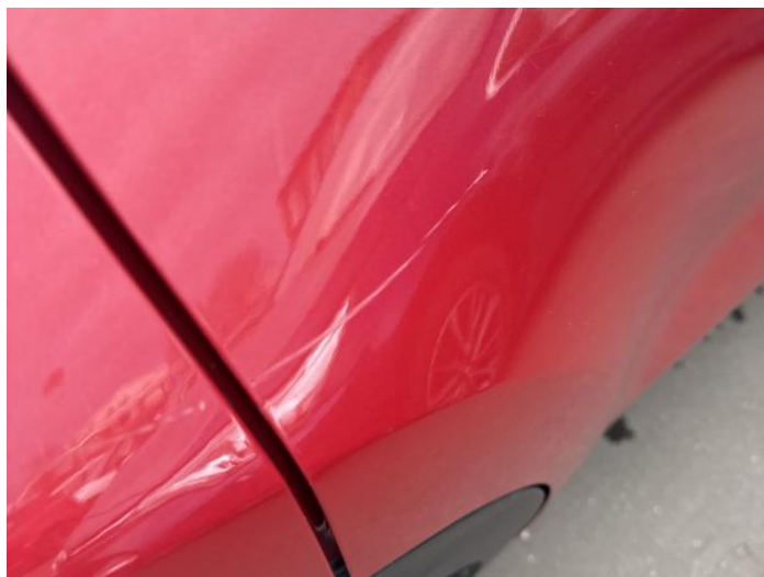
16: Door osr Scratched Over 25mm Thru Paint
