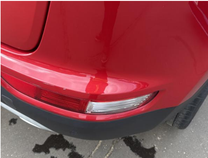
11: Bumper Rear Scratched 25 to 100mm Thru Paint
