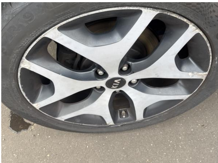
15: Wheel osr Scratched Over 50mm
