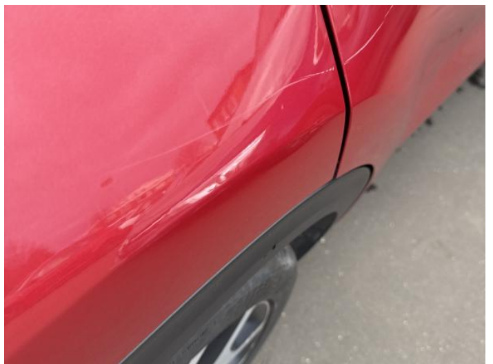
14: Qtr Panel osr Scratched Over 25mm Thru Paint
