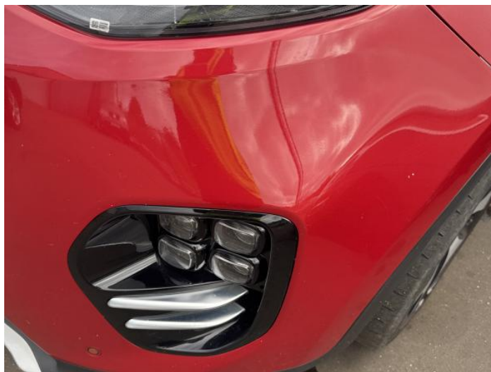
2: Bumper Front Poor Previous Repair Poor Paint
