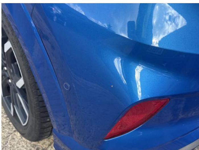
7: Bumper Rear Scratched 25 to 100mm Thru Paint
