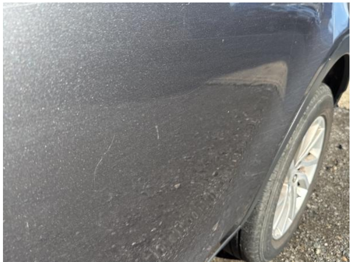
18: Door nsr Chipped Multiple Chips
