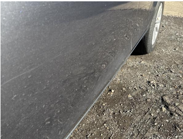
17: Door nsf Chipped Multiple Chips
