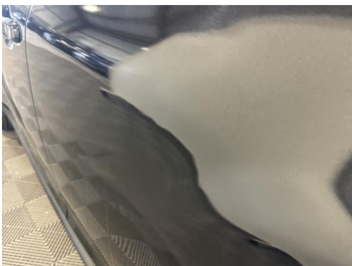
5: Door nsr Poor Previous Repair Poor Paint
