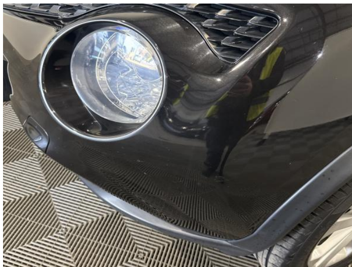
2: Bumper Front Scratched 25 to 100mm Thru Paint
