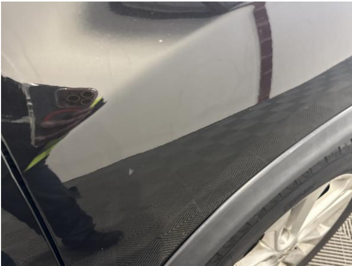
11: Wing osf Scratched UpTo 25mm Thru Paint
