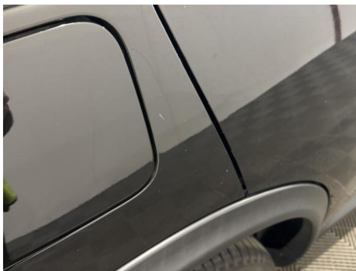
8: Qtr Panel osr Scratched UpTo 25mm Thru Paint
