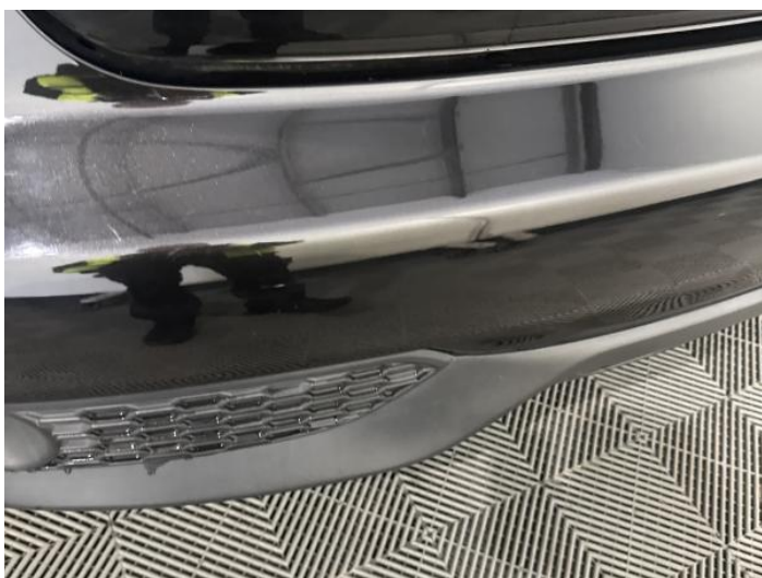
7: Bumper Rear Scratched 25 to 100mm Thru Paint
