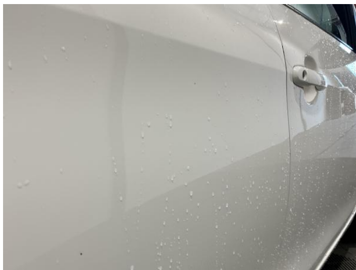
12: Door osr Poor Previous Repair Poor Paint
