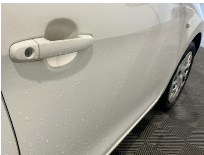
13: Door osf Poor Previous Repair Poor Paint
