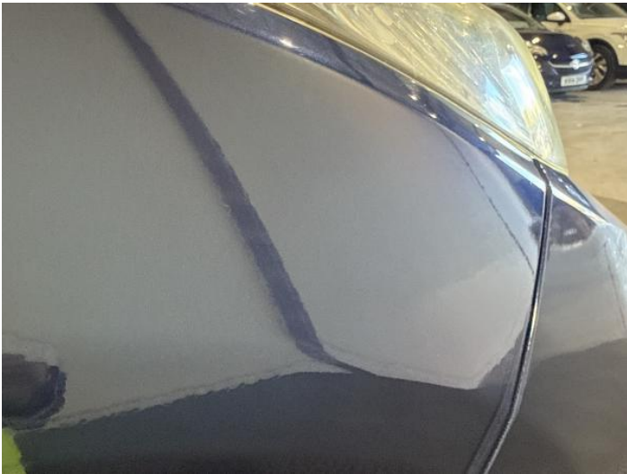
17: Wing osf Poor Previous Repair Poor Paint
