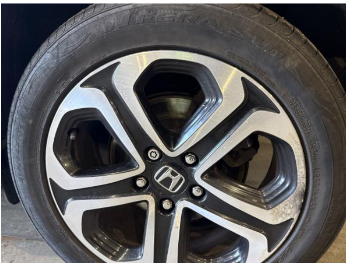
7: Wheel nsr Corroded Light
