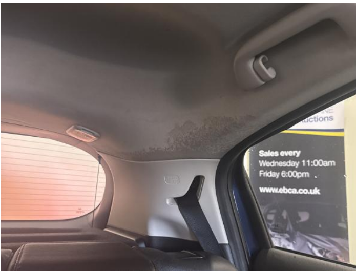
11: Roof Lining Soiled Light
