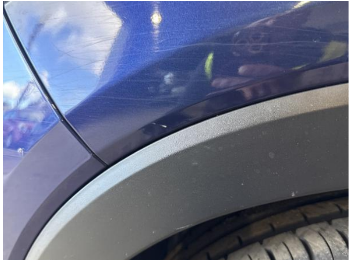
4: Wing nsf Scratched UpTo 25mm Thru Paint
