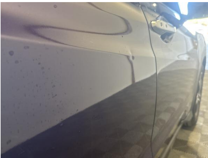
13: Door osr Dented Over 30mm
