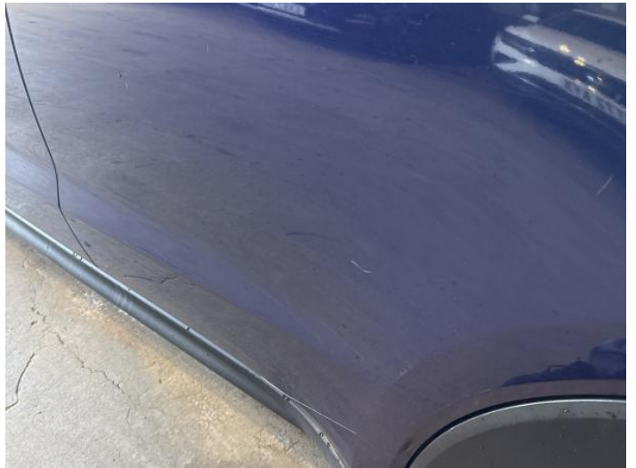
6: Door nsr Scratched Over 25mm Thru Paint
