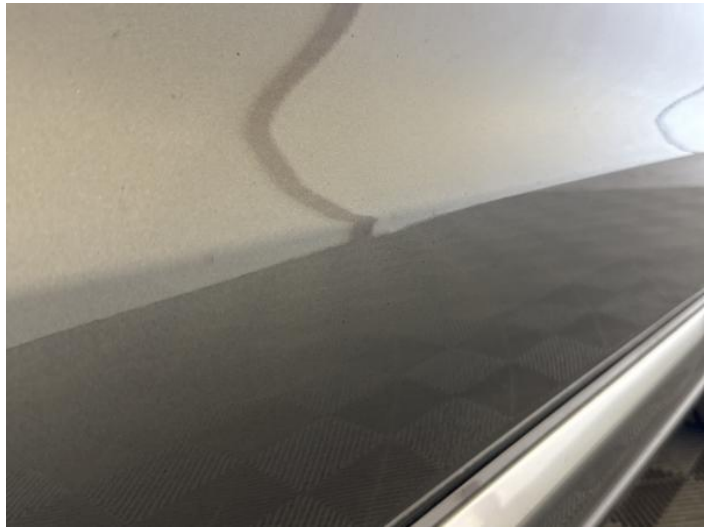
12: Door osf Dented Over 2 UpTo 10mm
