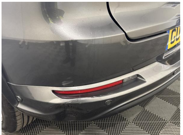
8: Bumper Rear Dented With Paint Damage
