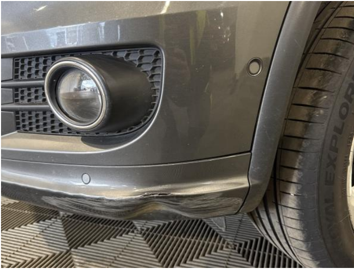
3: Bumper Front Cracked Over 25mm
