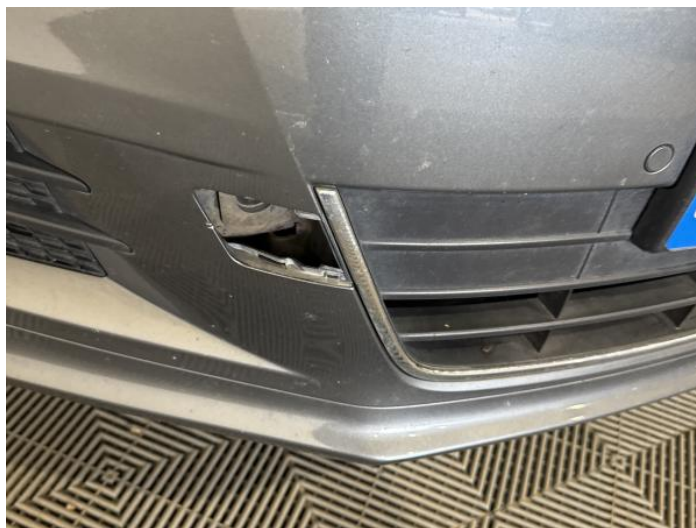
2: Front TowEye Cvr Missing Replace
