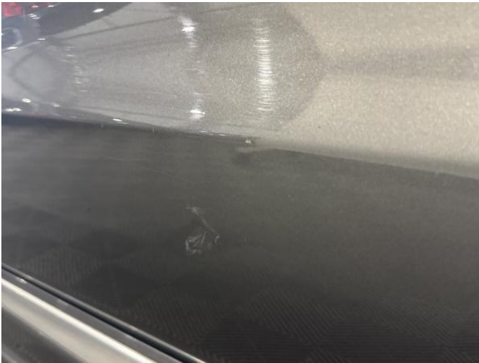
5: Door osf Dented With Paint Damage
