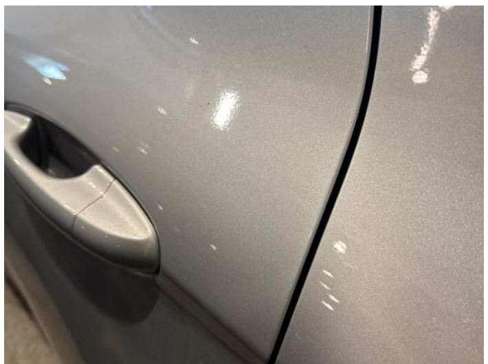
6: Door nsr Scratched UpTo 25mm Thru Paint
