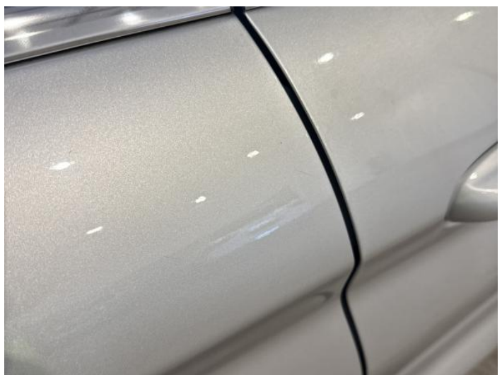
8: Door osr Scratched UpTo 25mm Thru Paint
