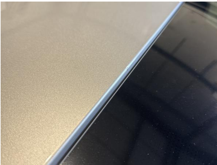
11: Roof Chipped Edge Chip
