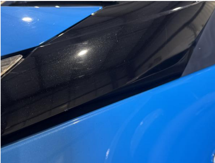
5: Wing nsf Scratched Over 25mm Thru Paint
