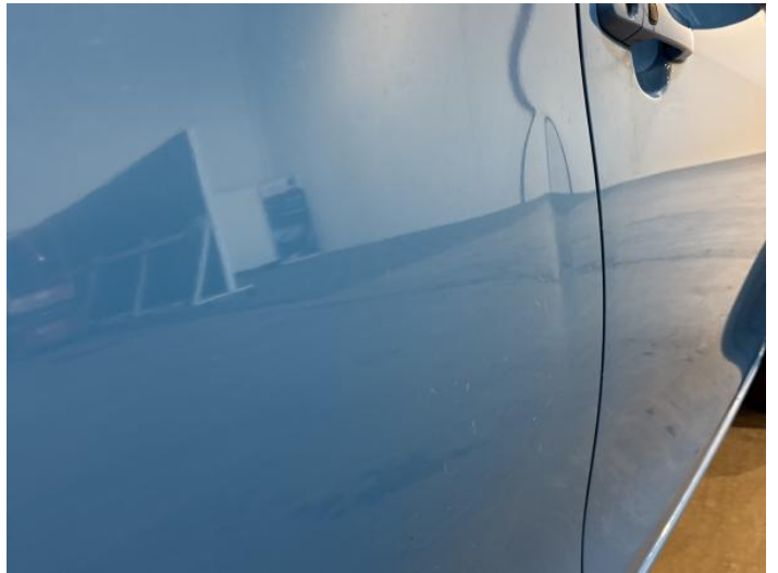
12: Door osr Dented Over 30mm
