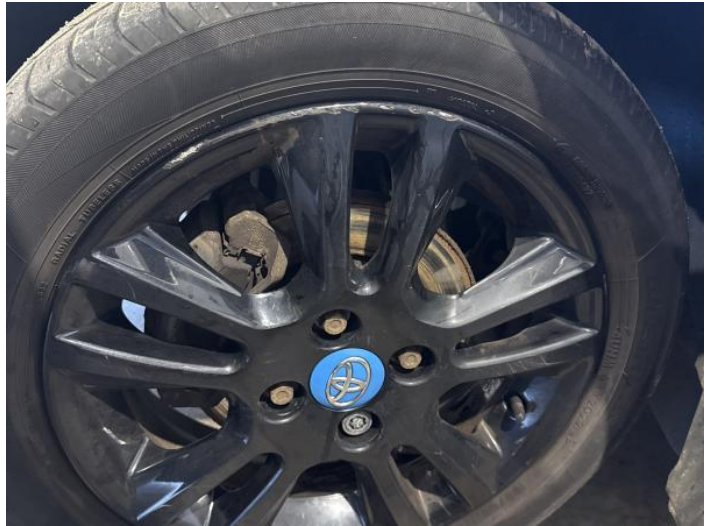
4: Wheel nsf Scratched Over 50mm
