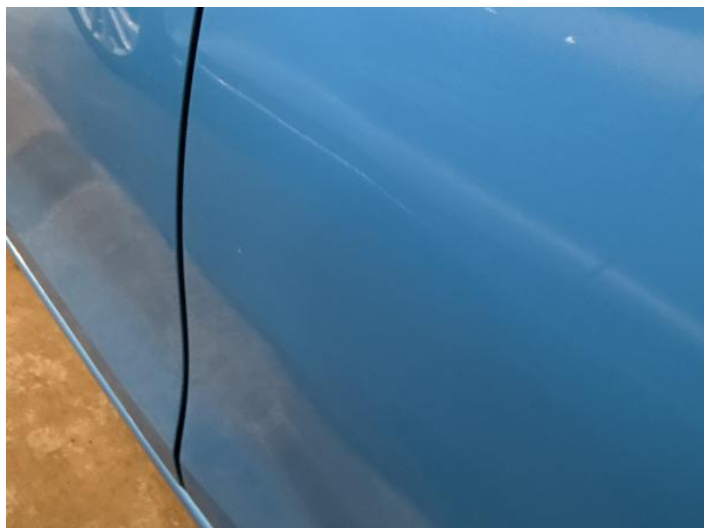
8: Door nsr Dented Over 30mm
