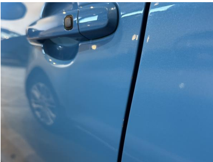
7: Door nsf Chipped Edge Chip
