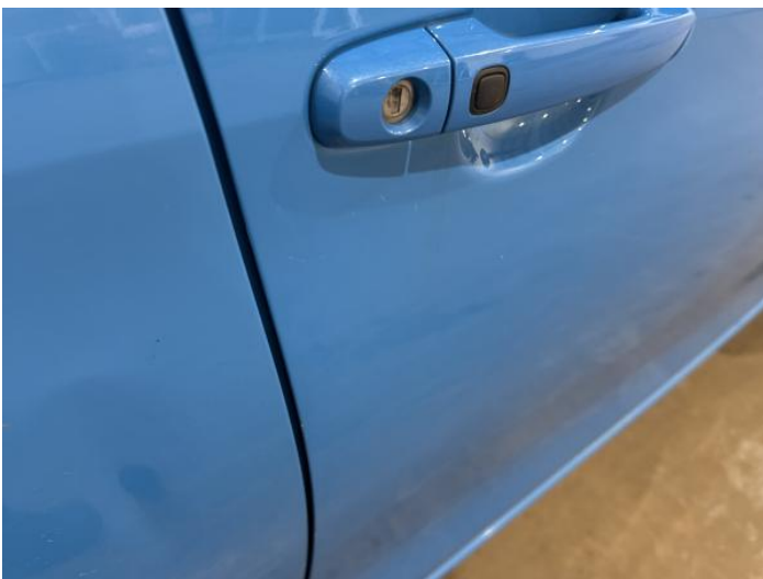
13: Door osf Chipped Edge Chip
