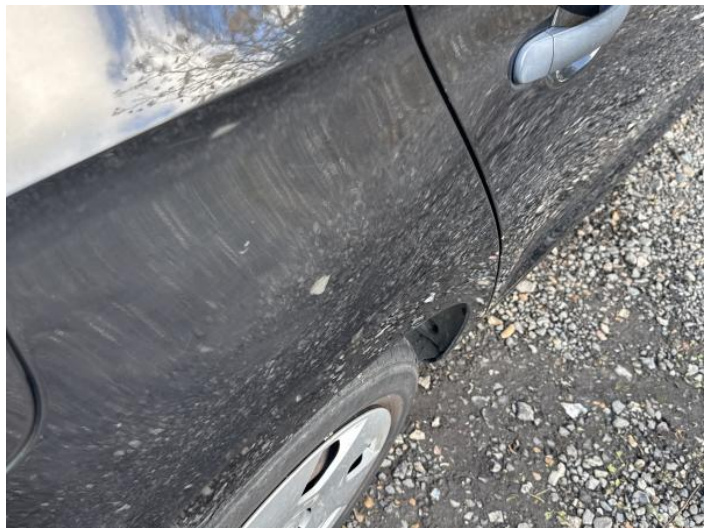
2: Qtr Panel or Chipped Multiple Chips
