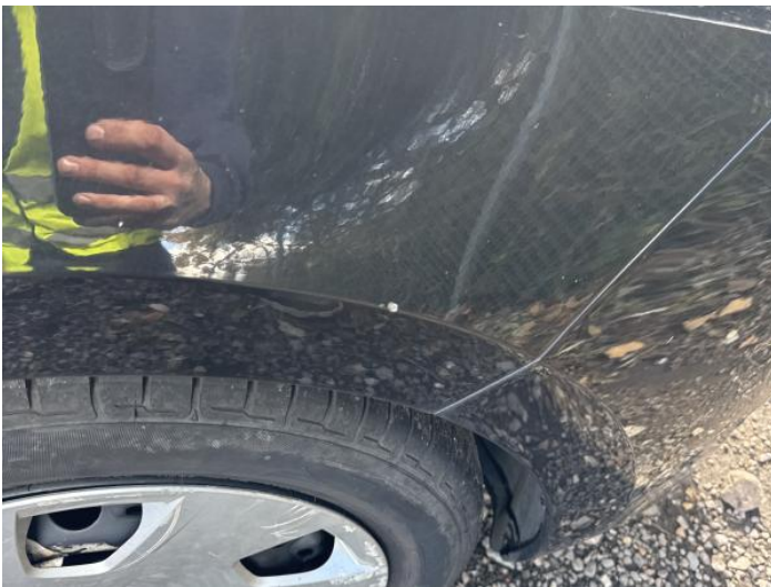
5: Wing osf Chipped Multiple Chips
