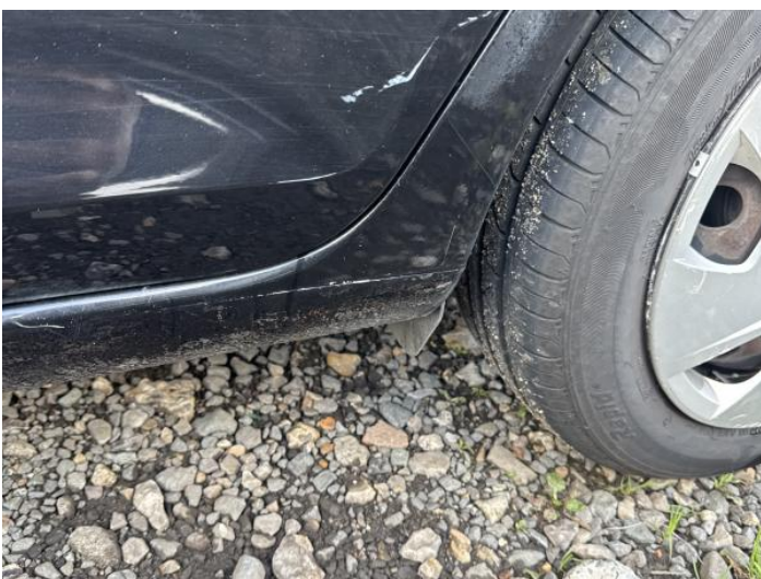
13: Sill ns Scratched UpTo 25mm Thru Paint
