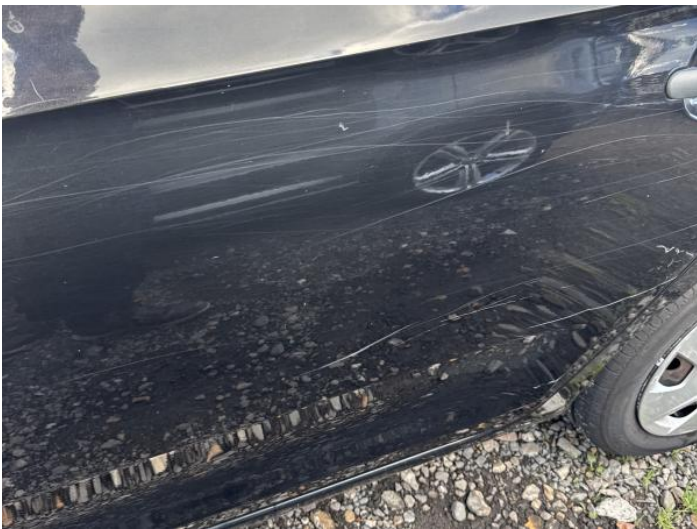
11: Door nsr Scratched Over 25mm Thru Paint
