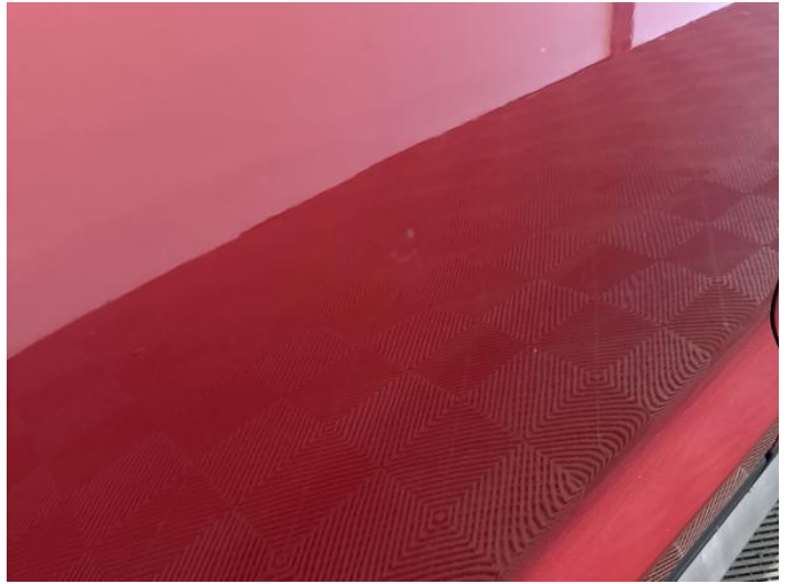
10: Door osr Dented Between 10mm + 30mm
