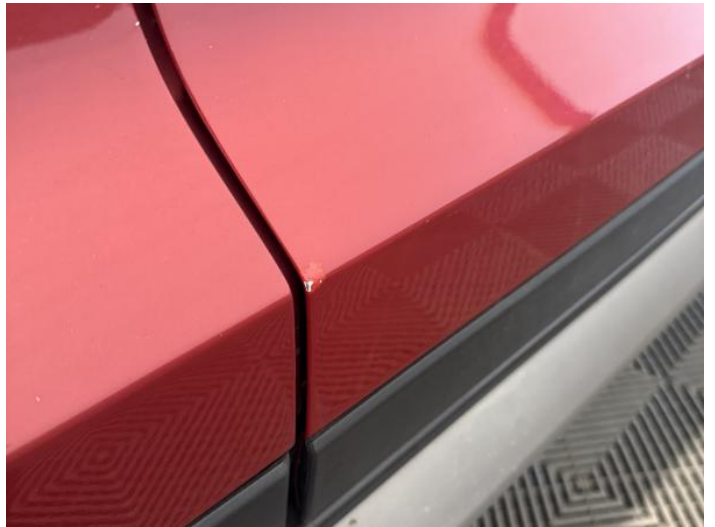
12: Door osf Scratched UpTo 25mm Thru Paint
