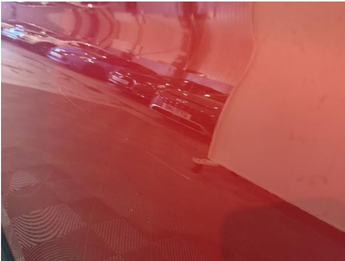
5: Door nsf Scratched Over 25mm Thru Paint
