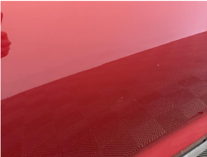
11: Door osr Scratched UpTo 25mm Thru Paint
