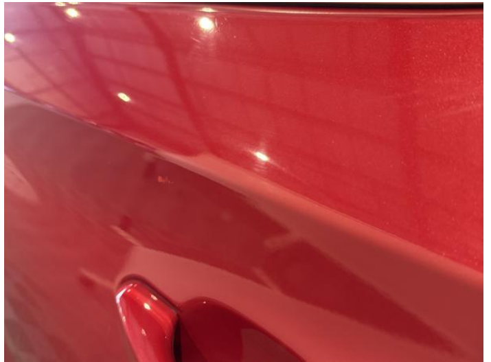
6: Door nsr Scratched UpTo 25mm Thru Paint
