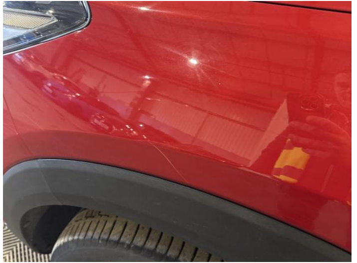
4: Wing nsf Scratched Over 25mm Thru Paint
