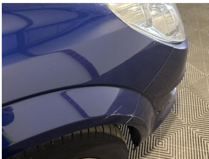
12: Wing osf Scratched Over 25mm Thru Paint
