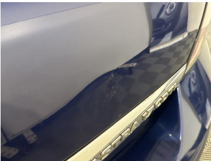
7: Tailgate Dented Over 30mm
