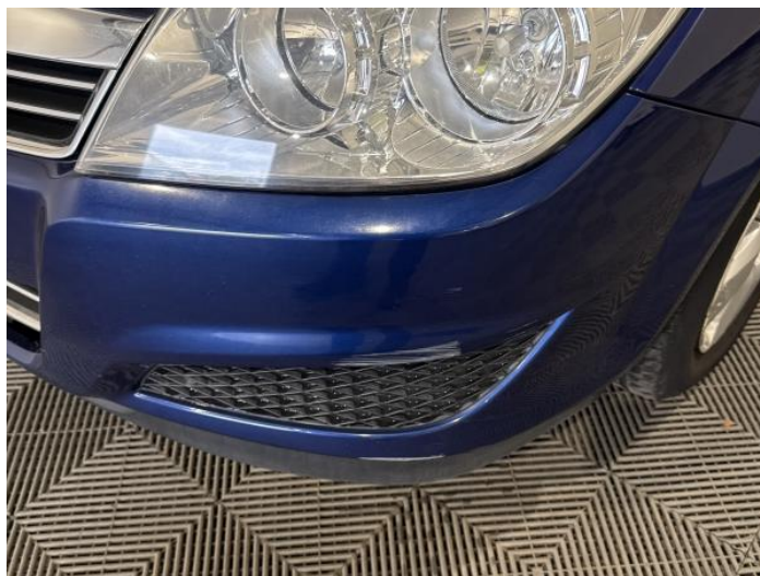
2: Bumper Front Scratched Over 100mm Thru Paint
