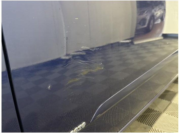
4: Door nsf Dented With Paint Damage
