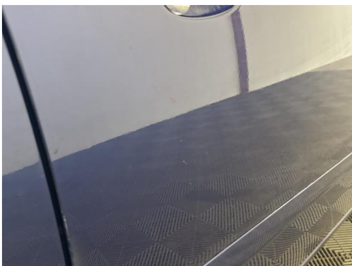
11: Door osf Scratched Over 25mm Thru Paint
