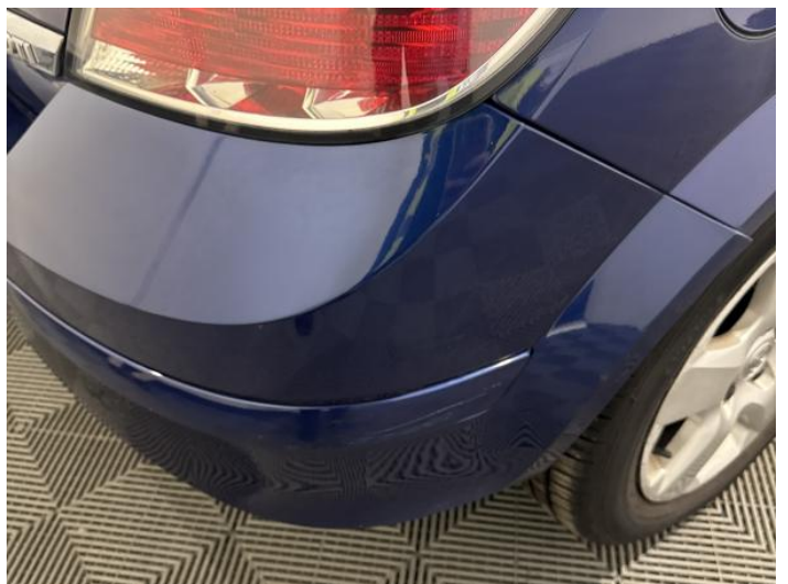
8: Bumper Rear Scratched 25 to 100mm Thru Paint
