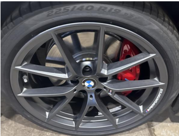
5: Wheel nsf Scratched Up To 50mm
