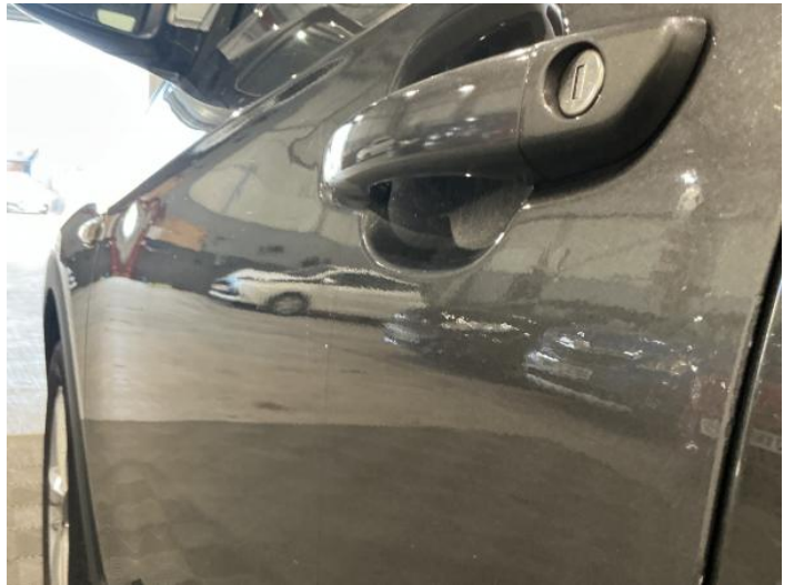
6: Door nsf Poor Previous Repair Poor Paint
