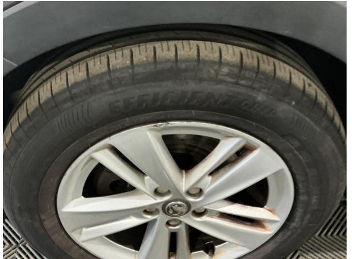
4: Wheel nsf Scratched Over 50mm
