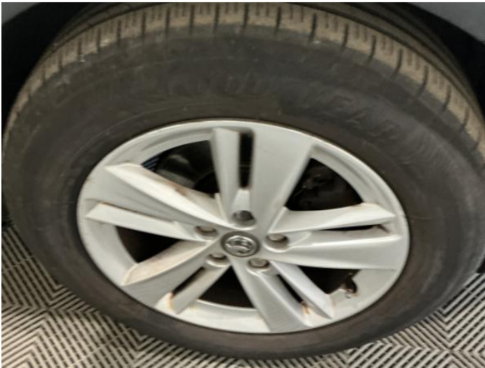
23: Wheel osf Scratched Over 50mm
