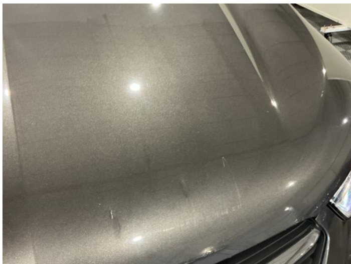
1: Bonnet Dented With Paint Damage
