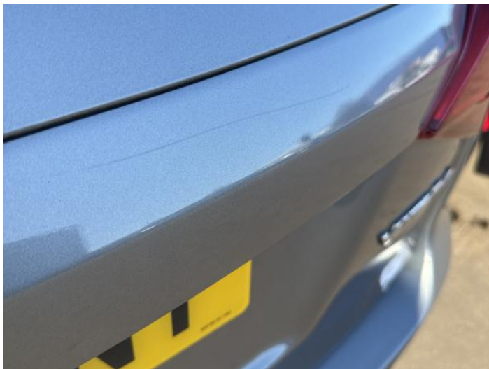
3: Boot Lid Scratched Over 25mm Thru Paint
