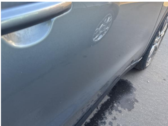
9: Door osf Dented With Paint Damage
