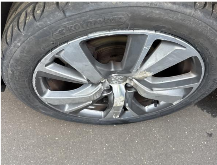
5: Wheel nsf Scratched Over 50mm
