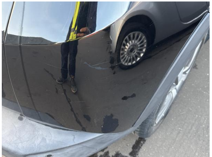
12: Bumper Rear Scratched 25 to 100mm Thru Paint
