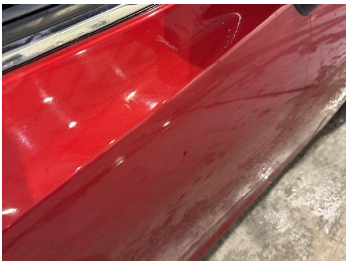
19: Door osr Poor Previous Repair Poor Paint
