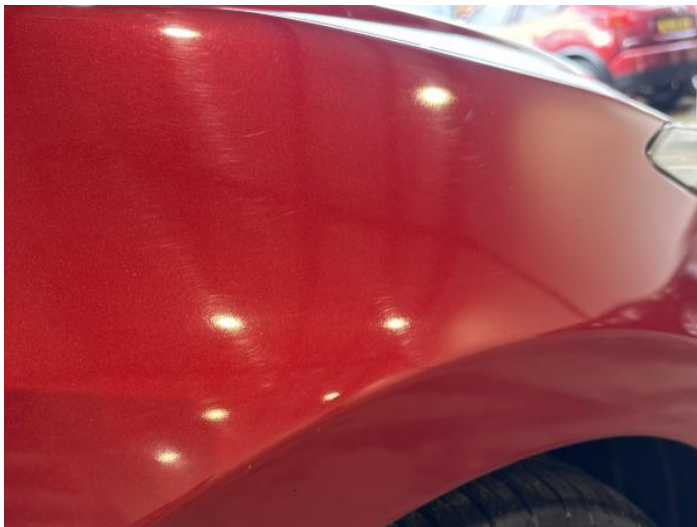
21: Wing osf Poor Previous Repair Poor Paint
