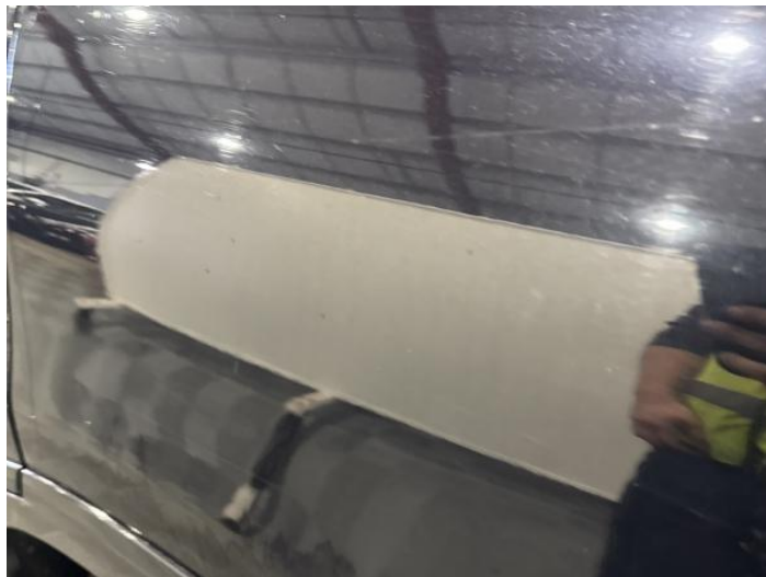
12: Qtr Panel nsr Dented Over 2 UpTo 10mm
