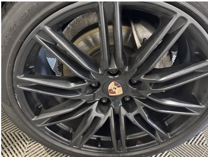
27: Wheel of Scratched Over 50mm
