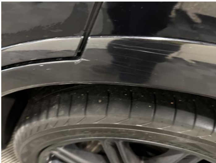
11: Qtr Panel Arch Extension ns Scratched (Painted) Over 25mm Thru Paint
