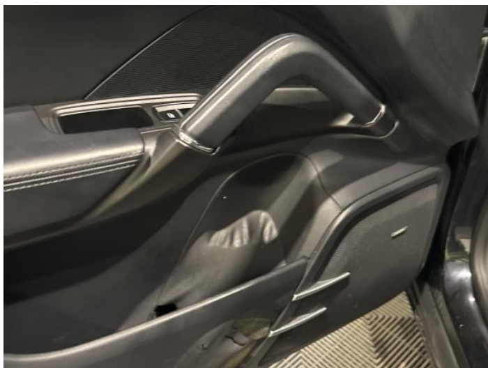
1: Door Pad nsf Torn Over 10mm
