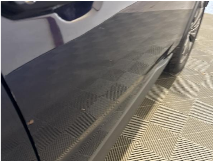
17: Door osf Dented Over 30mm
