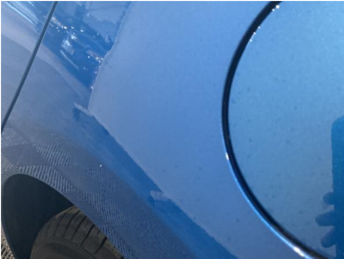
9: Qtr Panel nsr Dented Over 2 UpTo 10mm
