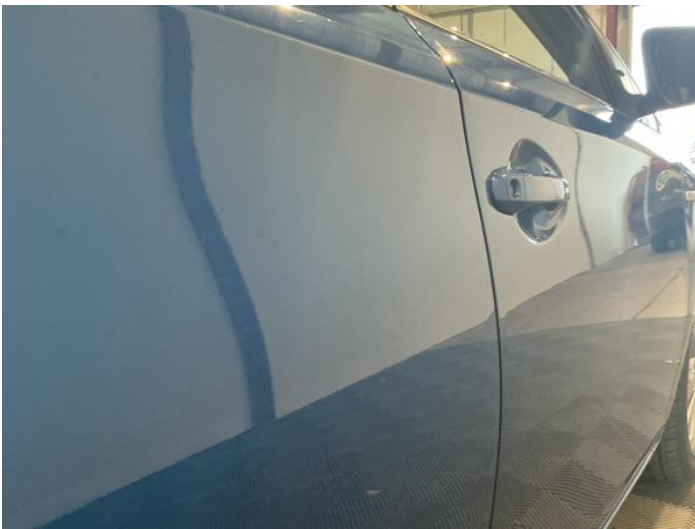
17: Door osr Dented Between 10mm + 30mm
