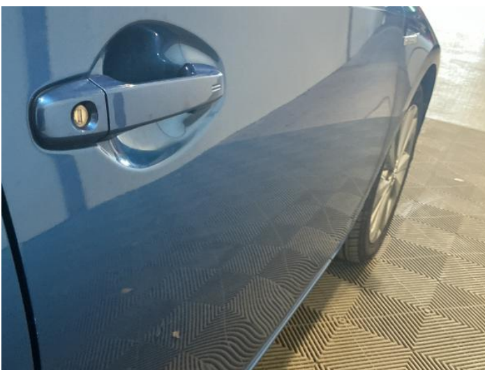
19: Door osf Poor Previous Repair Poor Paint
