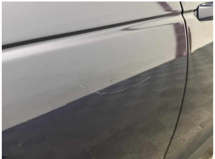
10: Door osr Scratched Over 25mm Thru Paint
