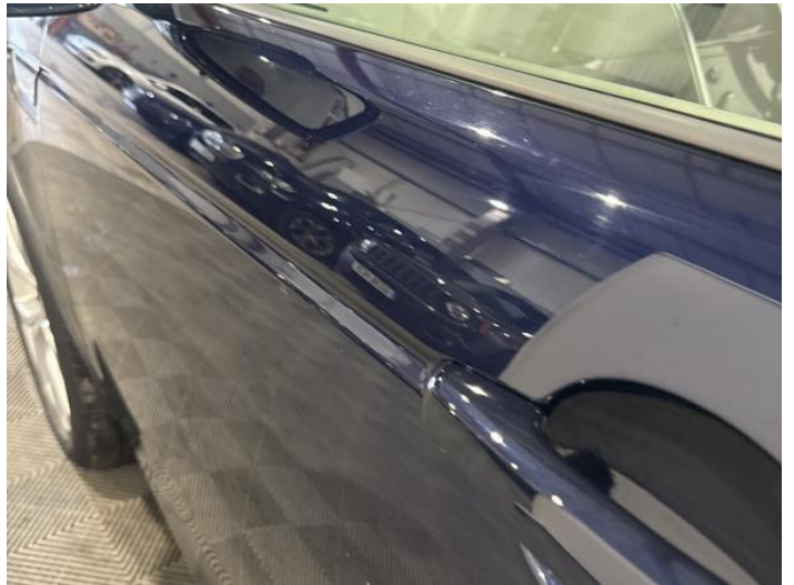
6: Door nsf Dented Between 10mm + 30mm
