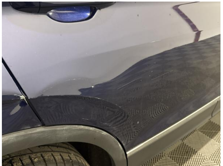
12: Door osr Dented With Paint Damage
