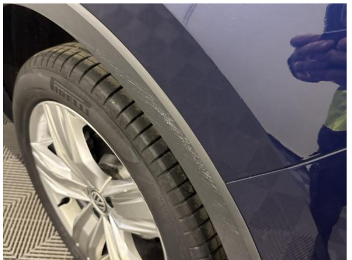
8: Qtr Panel Arch Extension ns Scuffed (Unpainted) UpTo 100mm
