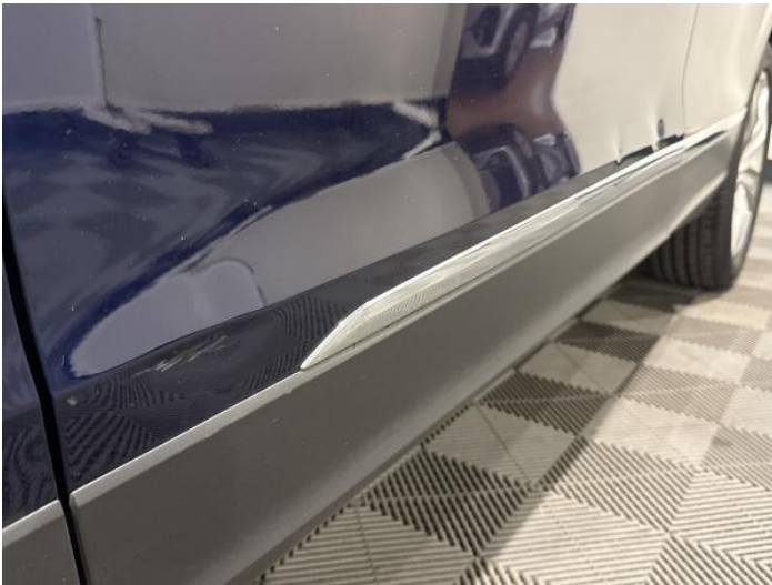
5: Door nsf Dented With Paint Damage
