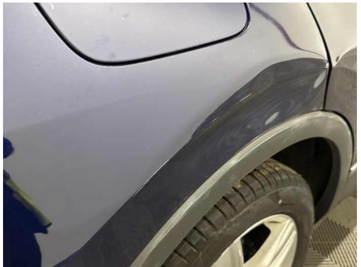
10: Qtr Panel osr Dented Over 30mm
