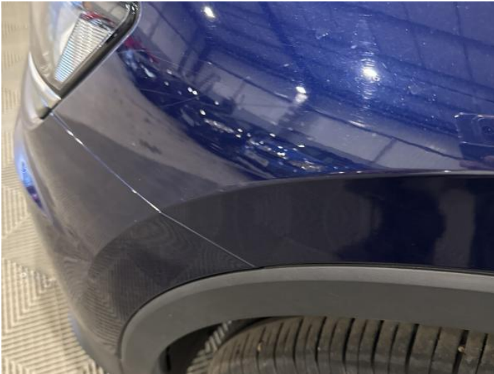
3: Wing nsf Scratched UpTo 25mm Thru Paint
