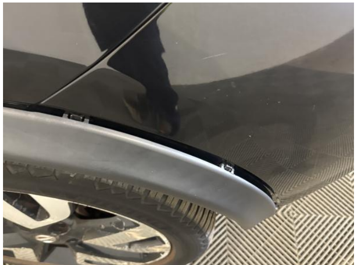
24: Wing Front Arch Extension os Broken Replace
