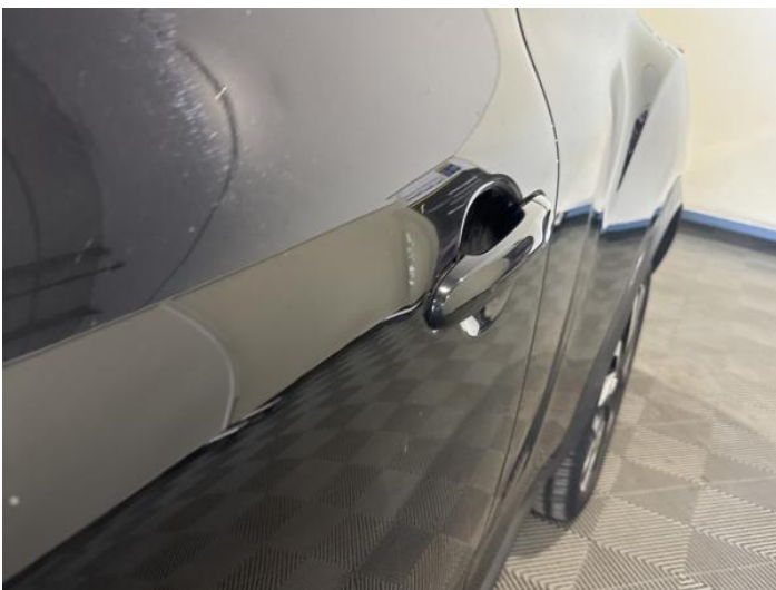
7: Door nsf Dented With Paint Damage
