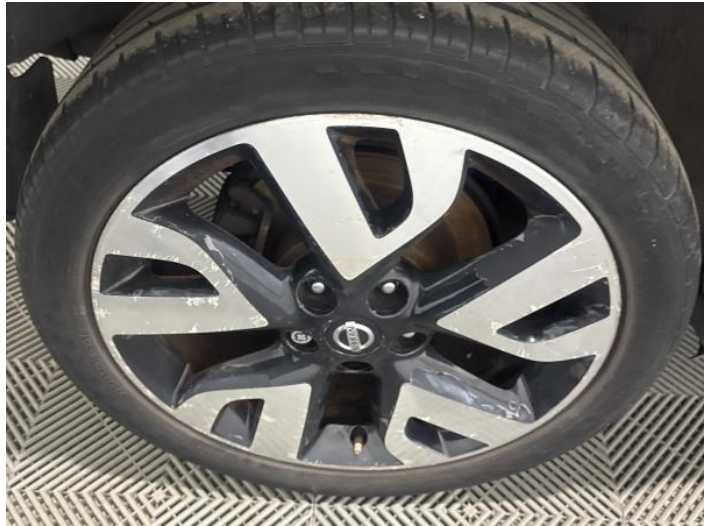
16: Wheel osf Scratched Over 50mm
