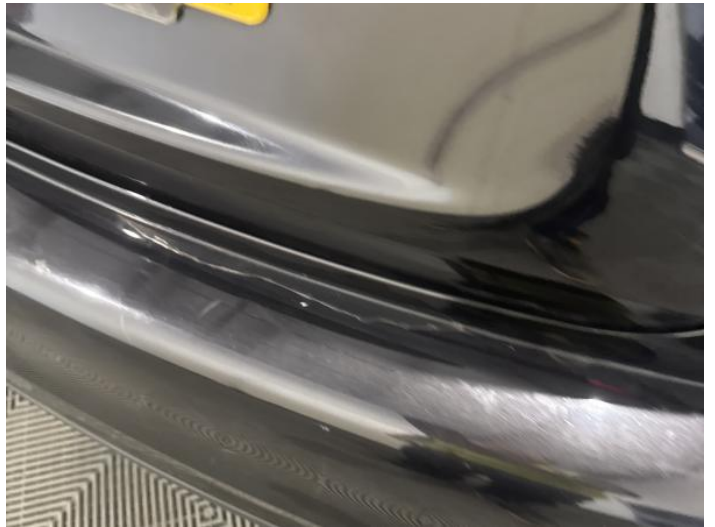
12: Bumper Rear Poor Previous Repair Paint Flake
