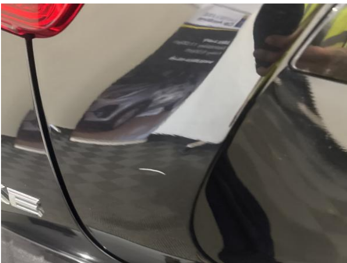
13: Boot Lid Scratched Over 25mm Thru Paint
