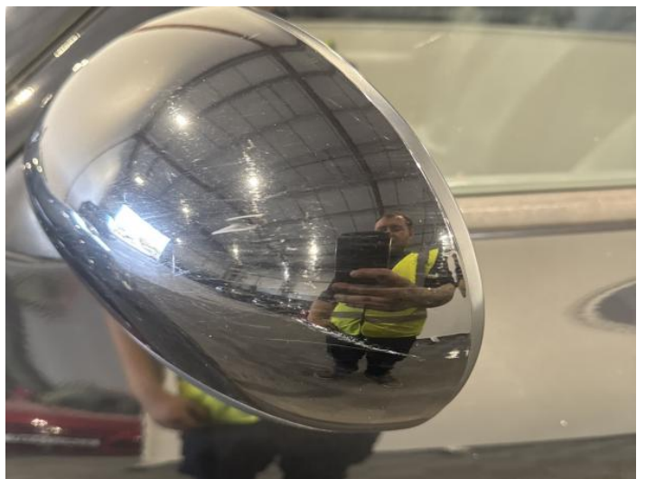
8: Door Mirror Assy nsf Scratched (Painted) Over 25mm Thru Paint
