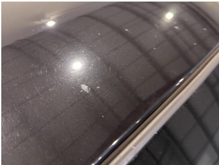
23: Roof Rusted UpTo 5mm
