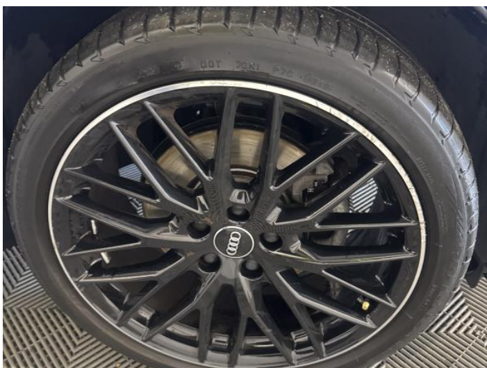
19: Wheel osf Scratched Over 50mm
