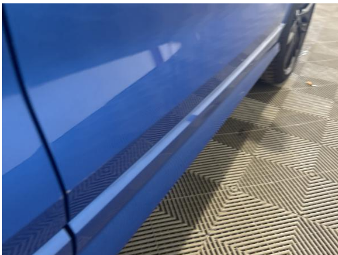
16: Door osf Scratched Over 25mm Thru Paint
