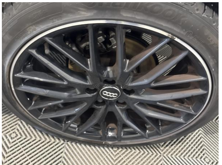
8: Wheel nsr Scratched Up To 50mm
