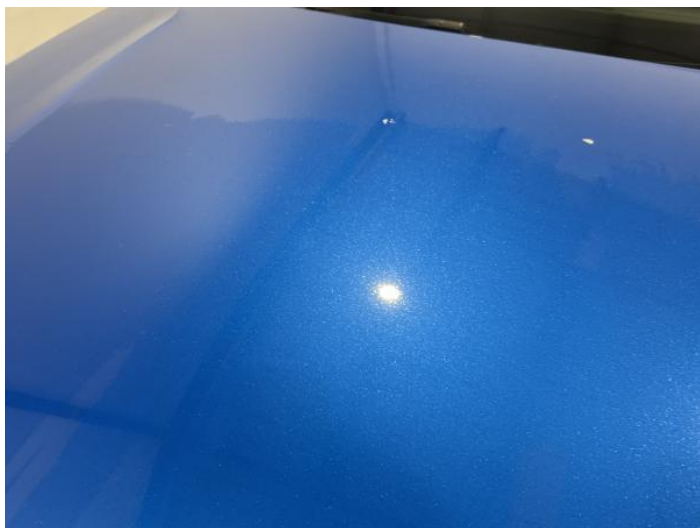
1: Bonnet Poor Previous Repair Paint Flake
