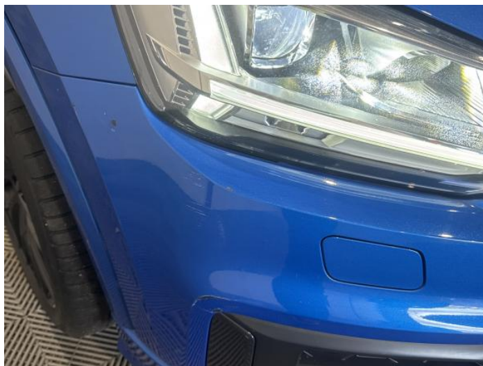
2: Bumper Front Scratched Over 100mm Thru Paint
