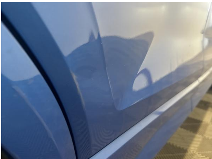
15: Door osr Dented With Paint Damage
